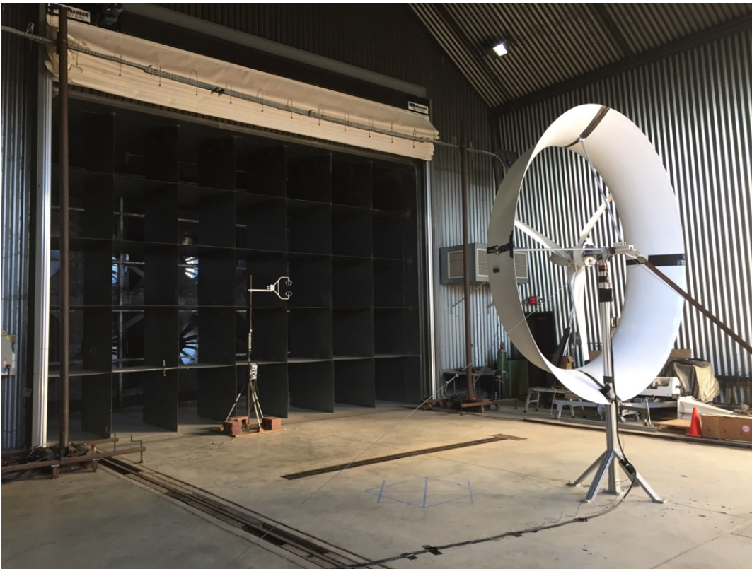
Figure 12: Ducted Rotor Under Test Conditions.
