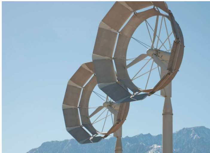
Figure 2: Commercial Attempts at Large Ducted Turbines a) Vortec 7 b) Ogin (FloDesign)
