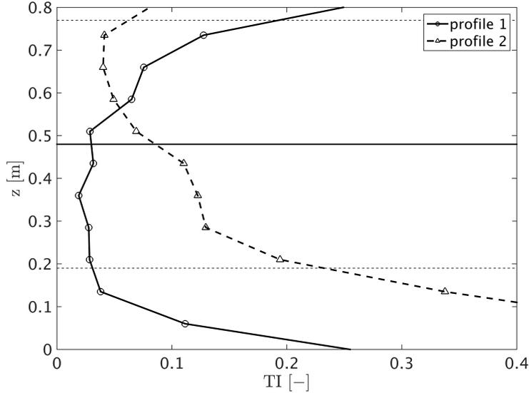
**Figure 2.** Turbulence intensities TI over height  $z$  for the respective mean values shown in Figure 1 of the manuscript.
