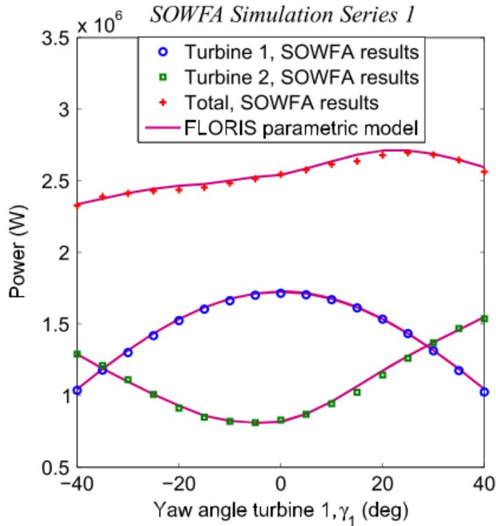
Figure 4. Screenshot taken from [4], Fig. 2, showing the power of an upstream turbine (blue), a downstream turbine (green, distance: 7D) and the total power of both (red) over the yaw angle of the upstream turbine.
