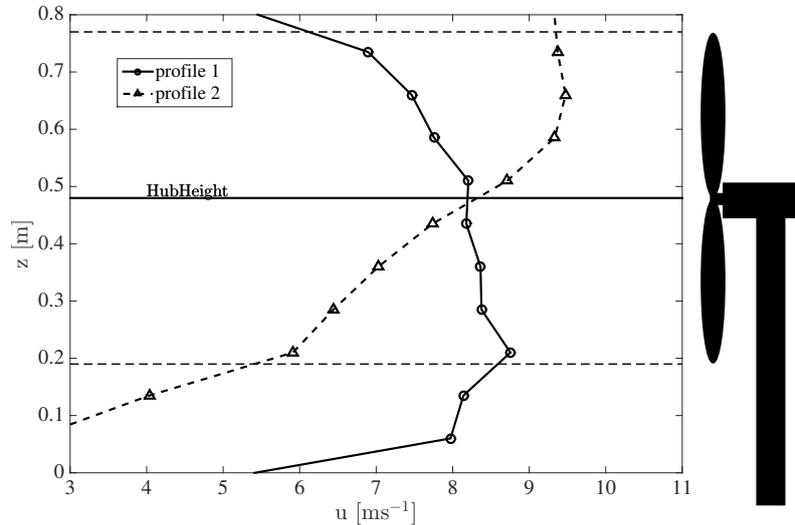
**Figure 1.** Mean velocity values of the vertical wind speed profiles 1 and 2 that were used as inflow conditions. The dashed, vertical lines mark the heights of the rotor tips of the turbine that was installed after characterizing the inflow profiles.
