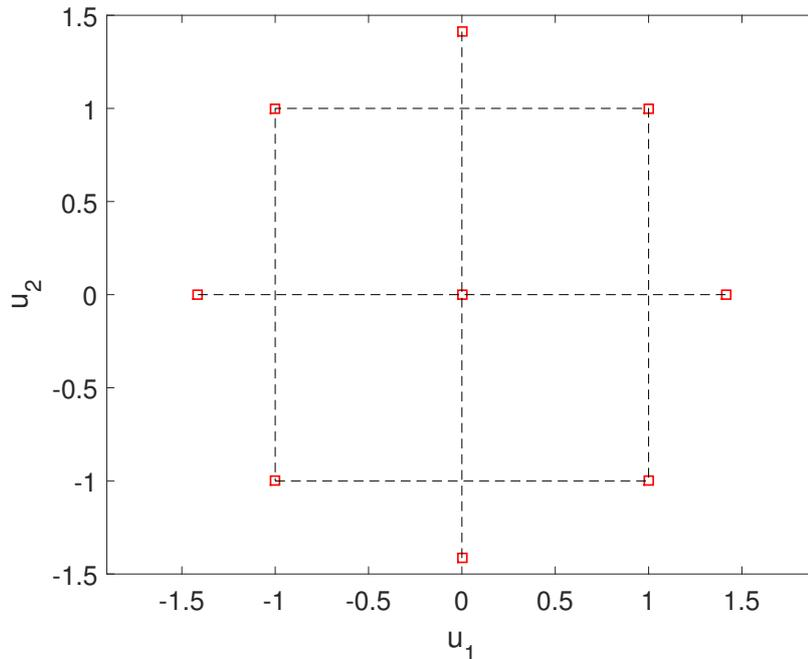
**Figure 11.** Example of a rotatable Central Composite Design (CCD) in a 2-dimensional standard Normal space  $[u_1, u_2]$ . The CCD consists of a central point, a  $2^k$  factorial design with 2 levels and  $k = 2$  dimensions, and axial points at distance  $u = \sqrt{2}$ , meaning that all the outer points lie on a circle.
