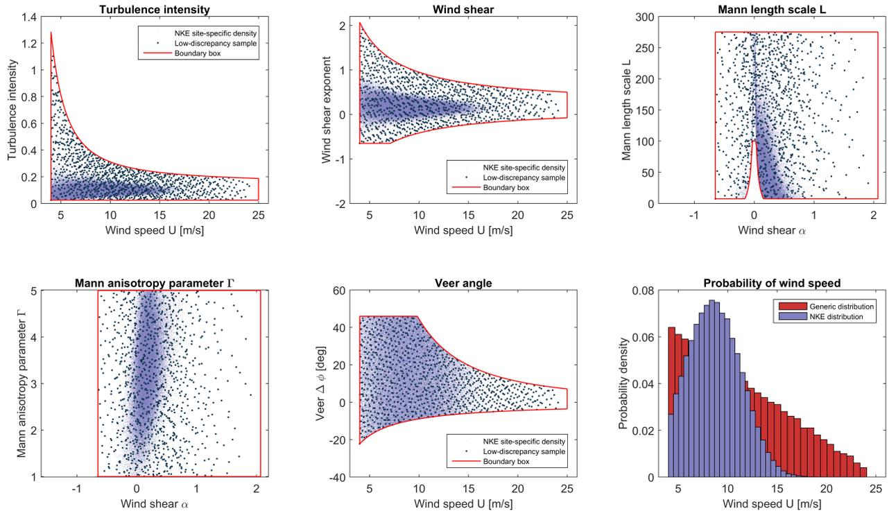
**Figure 2.** Sample distributions obtained using 1024 low-discrepancy points within a 6-dimensional variable space  $\{U, I_u, \alpha, \Delta\phi_h, L, \Gamma\}$ . Here  $U$  is Beta-distributed, while the other variables are uniformly distributed within their ranges. Blue shading shows the site-specific variable distribution for the NKE reference site (site 0, c.f. Table 2/Section 3).
