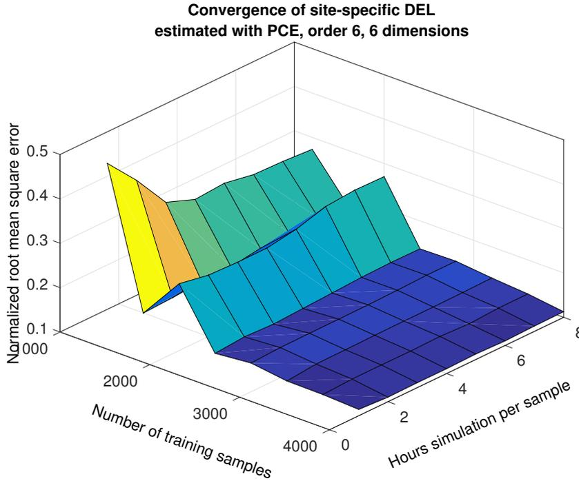
**Figure 10.** Convergence of a PCE of dimension 6 and order 6, as function of number of collocation points and hours of simulation per collocation point. The z-axis represents the NRMS error obtained from the difference between 500 site-specific pseudo-MC samples of blade root flapwise DEL for reference site 0, and the corresponding predictions from PCE.
