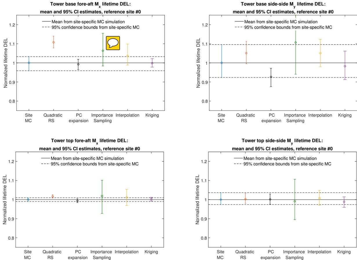
**Figure 13.** Comparison of predictions of the lifetime damage-equivalent loads for six different estimation approaches. All values are normalized with respect to the mean estimate from a site-specific Monte Carlo simulation.
