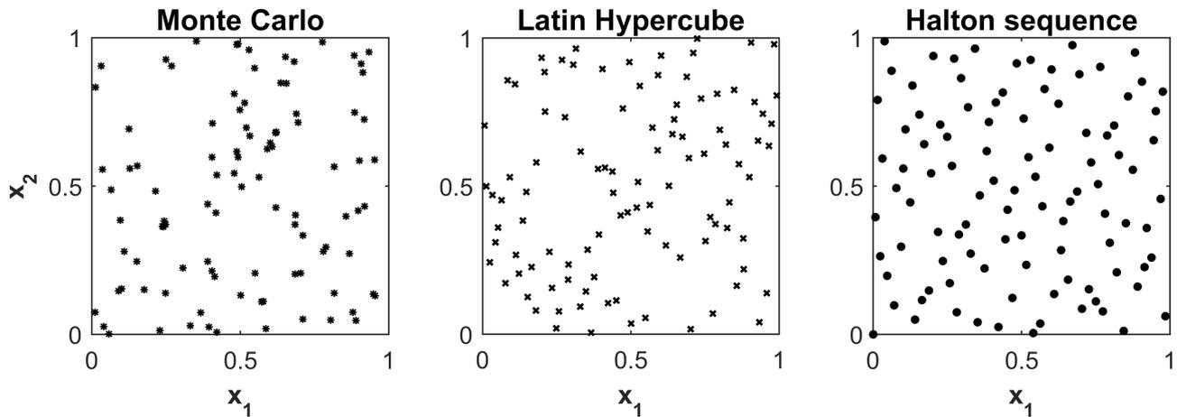
**Figure 1.** Comparison of several simulation-based experimental design approaches. Examples show random (Monte Carlo and Latin Hypercube) or pseudorandom (Halton sequence) samples of size 100 drawn from a uniform distribution within a unit hypercube.
