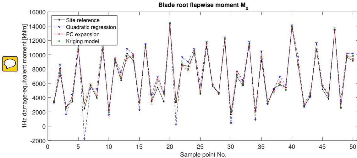
**Figure 15.** Sample-by-sample comparison of the 1Hz damage-equivalent load predictions, for two load prediction methods - quadratic Response Surface, and Polynomial Chaos expansion, compared against site-specific Monte Carlo simulation. Each point on the  $x$ -axis represents a sample point from the site-specific distribution of input variables for reference site 0, and the  $y$ -axis represents the estimated mean 1Hz-equivalent load.
