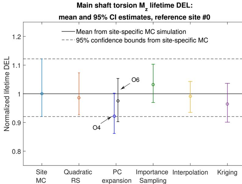
**Figure 12.** Comparison of predictions of the lifetime damage-equivalent loads for six different estimation approaches. All values are normalized with respect to the mean estimate from a site-specific Monte Carlo simulation, and the error bars represent the bounds of the 95% confidence intervals. Results from two PCEs are shown: the blue bar corresponds to the output of a 4<sup>th</sup> order PCE, while the black bar corresponds to a 6<sup>th</sup> order PCE.
