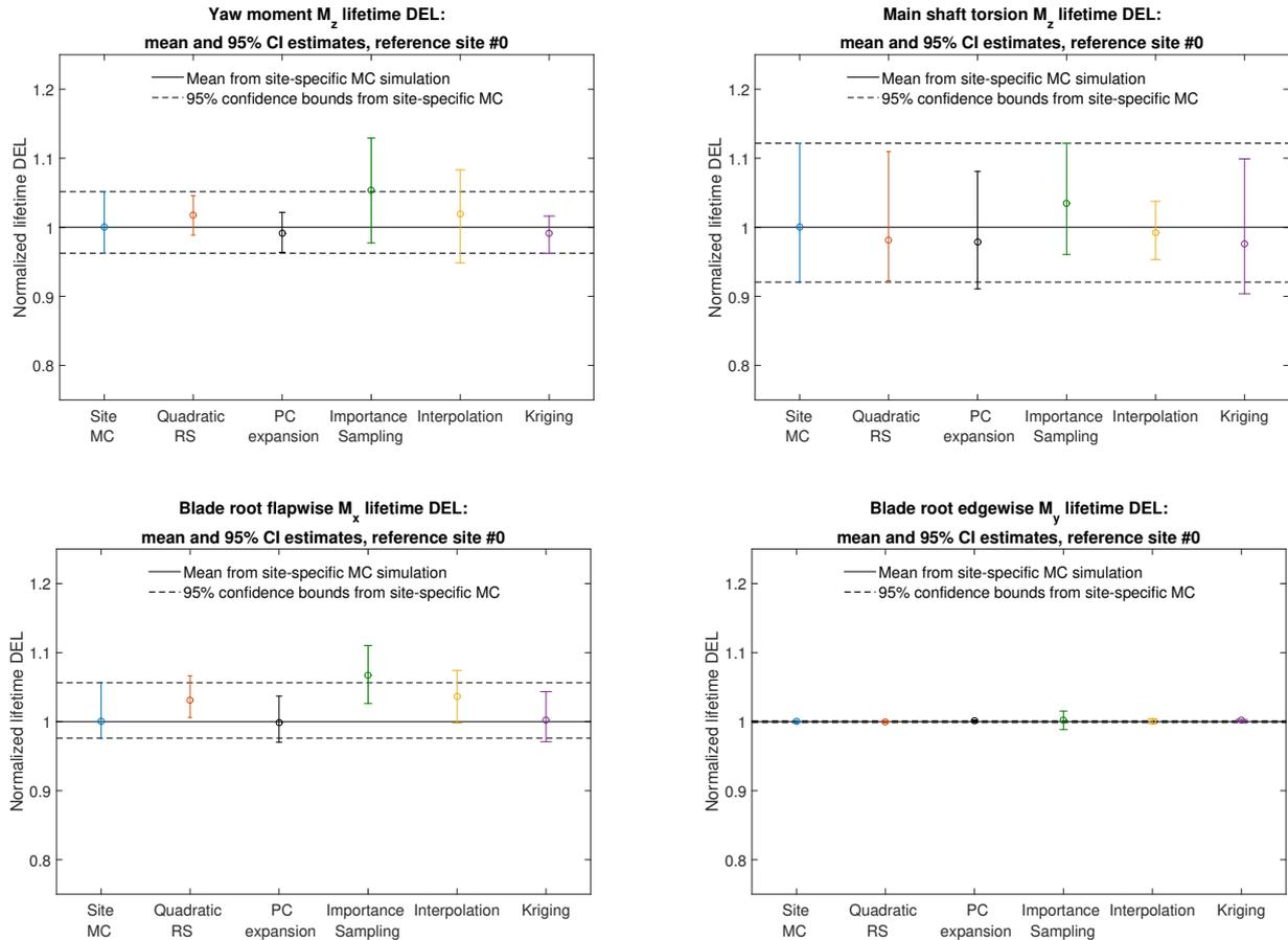
**Figure 14.** Comparison of predictions of the lifetime damage-equivalent loads for six different estimation approaches. All values are normalized with respect to the mean estimate from a site-specific Monte Carlo simulation.
