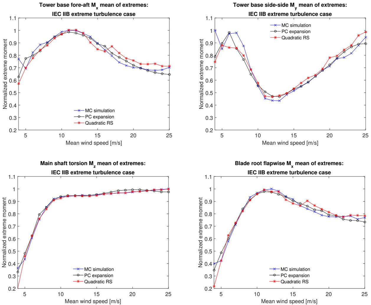
**Figure 16.** Comparison of predictions of the mean of extremes obtained for the extreme turbulence load case DLC1.3 for IEC turbulence class B conditions. MC simulation (blue lines with crosses) denotes the reference values obtained with full-fidelity aeroelastic simulations.
