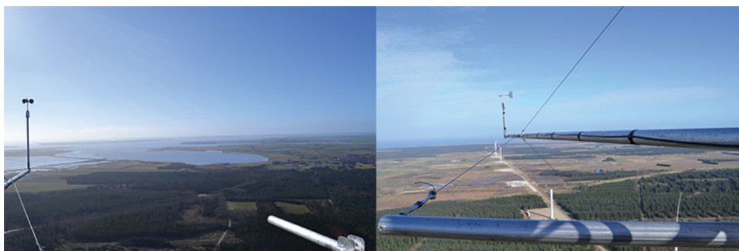
Figure 7. Left: Cup anemometer (left) and wind vane (right) at 244 m height, Østerild test site. Permissions by DTU Wind Energy.
