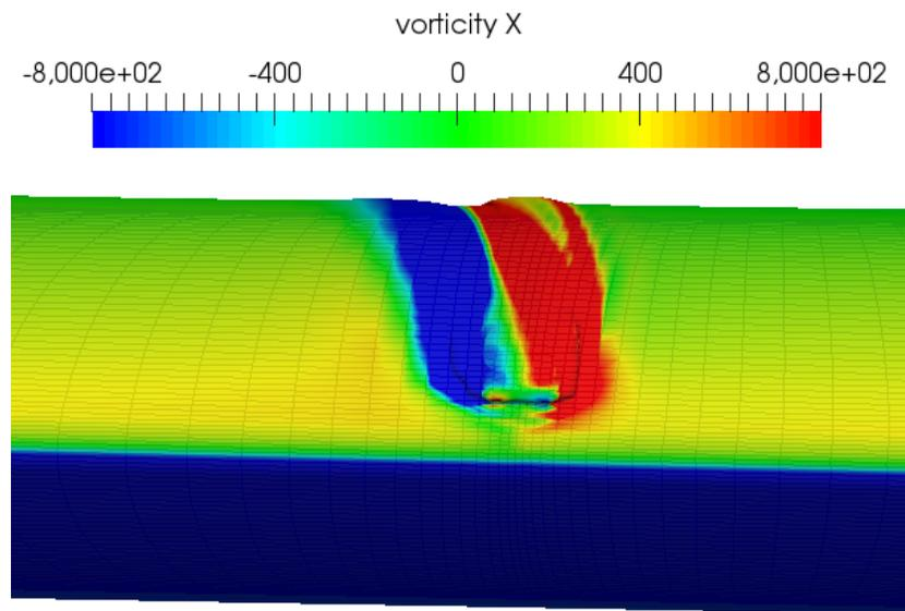
Figure 2: Iso-surface of the vorticity in the chordwise direction.
