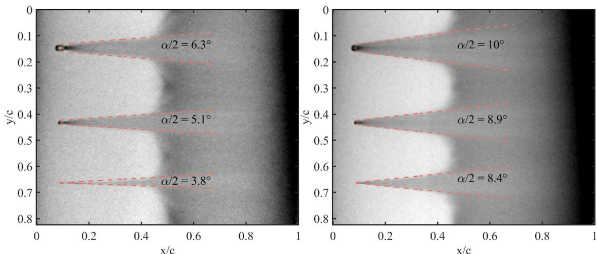
Figure 1: Estimation of spreading angles of turbulent wedges on a DU 91-W2-250 airfoil induced by turbulators ( $h \in [0.5; 1; 1.5] \text{ mm}$ ) for  $Re = 300,000$  (left) and  $Re = 600,000$  (right).
