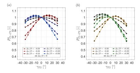
Figure 13. Combined relative power  $P_{T1+T2}^*$  of two turbines as a function of the downstream turbine yaw angle  $\gamma_{T2}$  for different lateral offset positions  $\Delta z/D$ . The upstream turbine yaw angle is kept constant at (a)  $\gamma_{T1}=0^\circ$  and (b)  $\gamma_{T1}=30^\circ$  respectively. The downstream turbine T2 is located at x/D=3. The turbines are exposed to inflow B.
