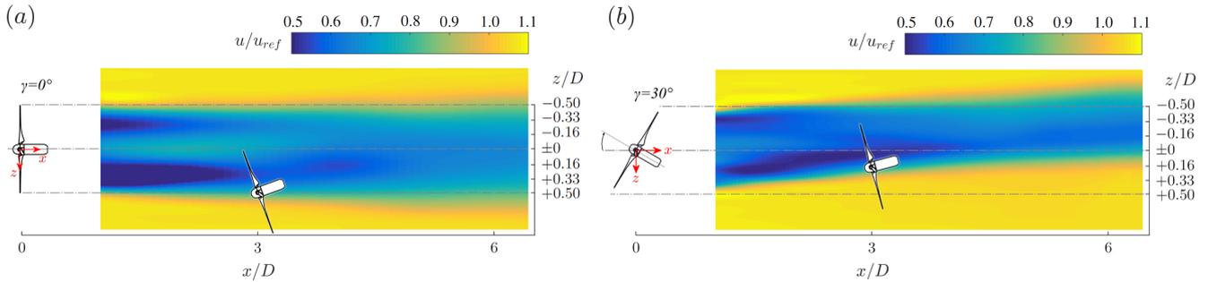
**Figure 10.** (a) Topview of the downstream turbine T2 operated at a lateral offset position  $\Delta z/D = +0.50$  and a yaw angle of  $\gamma_{T2} = -20^\circ$  in the wake of an upstream turbine T1 operated at  $\gamma_{T1} = 0^\circ$ . (b) Topview of the downstream turbine T2 operated at a lateral offset position ( $\Delta z/D = +0.16$ ) and a yaw angle of  $\gamma_{T2} = -15^\circ$  in the wake of an upstream turbine T1 operated at  $\gamma_{T1} = 30^\circ$ .
