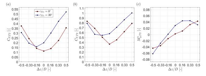
Figure 8. Downstream turbine (a) power coefficient, (b) thrust coefficient and (c) normalized yaw moment as a function of its lateral offset position  $\Delta z/D$ . The upstream turbine yaw angle is kept constant at  $\gamma_{T1} = 0^{\circ}$ . The downstream turbine T2 is located at x/D = 3. The turbines are exposed to inflow B.
