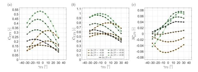
Figure 12. Downstream turbine (a) power coefficient, (b) thrust coefficient and (c) normalized yaw moment as a function of its yaw angle  $\gamma_{T2}$  for different lateral offset position  $\Delta z/D$ . The upstream turbine yaw angle is kept constant at  $\gamma_{T1}=30^{\circ}$ . The downstream turbine T2 is located at x/D=3. The turbines are exposed to inflow B.
