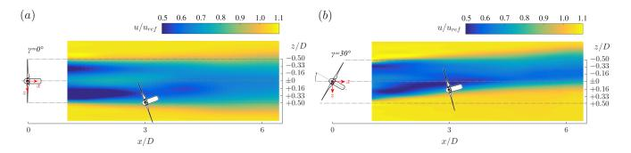
Figure 10. (a) Topview of the downstream turbine T2 operated at a lateral offset position  $\Delta z/D = +0.50$  and a yaw angle of  $\gamma_{T2} = -20^{\circ}$  in the wake of an upstream turbine T1 operated at  $\gamma_{T1} = 0^{\circ}$ . (b) Topview of the downstream turbine T2 operated at a lateral offset position  $(\Delta z/D = +0.16)$  and a yaw angle of  $\gamma_{T2} = -15^{\circ}$  in the wake of an upstream turbine T1 operated at  $\gamma_{T1} = 30^{\circ}$ .
