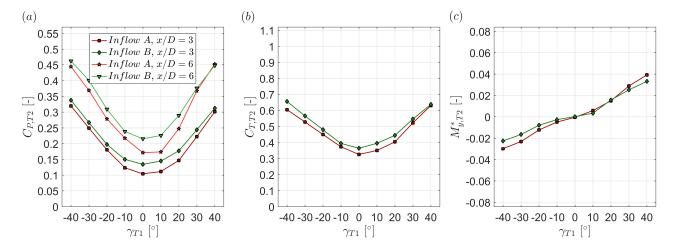
Figure 4. Downstream turbine (a) power coefficient, (b) thrust coefficient and (c) normalized yaw moment as a function of the upstream turbine's yaw angle  $\gamma_{T1}$ . The downstream turbine T2 is located at x/D=3 and x/D=6 respectively. The turbines are exposed to inflows A and B.
