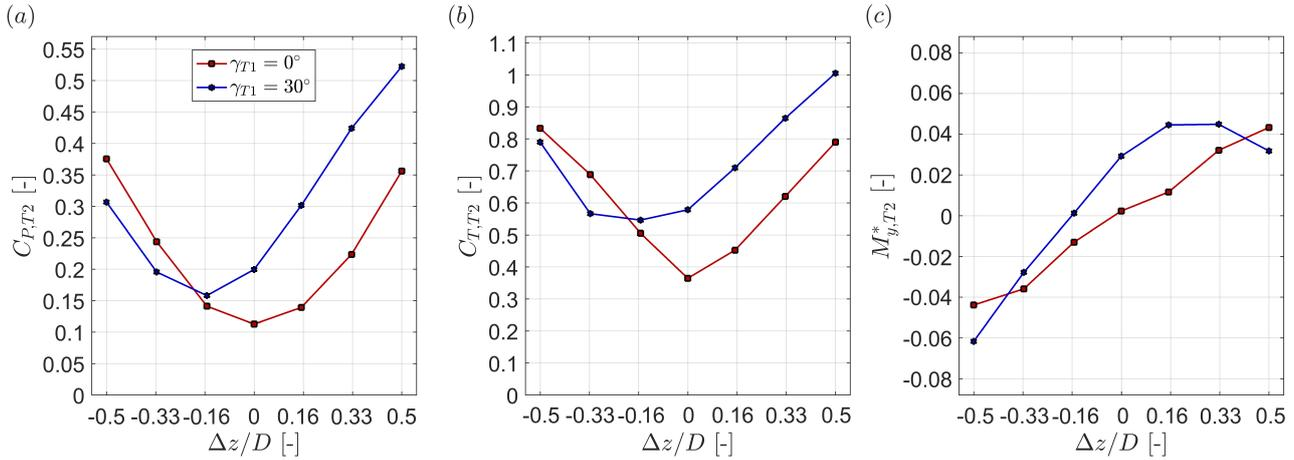
**Figure 8.** Downstream turbine (a) power coefficient, (b) thrust coefficient and (c) normalized yaw moment as a function of its lateral offset position  $\Delta z/D$ . The upstream turbine yaw angle is kept constant at  $\gamma_{T1} = 0^\circ$ . The downstream turbine T2 is located at  $x/D = 3$ . The turbines are exposed to inflow B.
