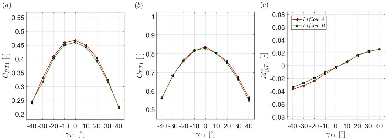
**Figure 1.** (a) Power coefficient  $C_{P,T1}$  (b) thrust coefficient  $C_{T,T1}$  and (c) normalized yaw moment  $M_{y,T1}^*$  of the undisturbed upstream turbine T1 for different inflow conditions. The turbine is operated at  $\lambda_{opt,T1} = 6.0$  for all yaw angles.
