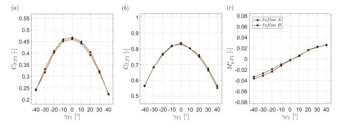
Figure 1. (a) Power coefficient  $C_{P,T1}$  (b) thrust coefficient  $C_{T,T1}$  and (c) normalized yaw moment  $M_{u,T1}^*$  of the undisturbed upstream turbine T1 for different inflow conditions. The turbine is operated at  $\lambda_{opt,T1} = 6.0$  for all yaw angles.
