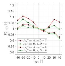
Figure 5. Combined relative power  $P_{T1+T2}^*$  of two turbines for different upstream turbine yaw angles  $\gamma_{T1}$ . The downstream turbine T2 is located at x/D=3 and x/D=6 respectively. The turbines are exposed to inflows A and B.
