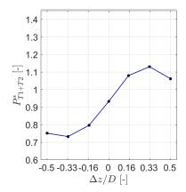
Figure 9. Combined relative power  $P_{T1+T2}^*$  of the two-turbine-array for different lateral offset positions  $\Delta z/D$ . The combined power is calculated for a change of upstream turbine yaw angle from  $\gamma_{T1}=0^\circ$  to  $+30^\circ$  for each position. The downstream turbine T2 is located at x/D=3. The turbines are exposed to inflow B.
