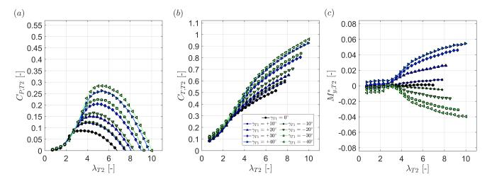
Figure 3. Downstream turbine (a) power coefficient, (b) thrust coefficient and (c) normalized yaw moment as a function of its tip speed ratio  $\lambda_{T2}$  for different upstream turbine yaw angles  $\gamma_{T1}$ . The downstream turbine T2 is located at x/D = 3. The turbines are exposed to inflow B.
