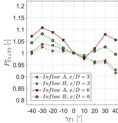
**Figure 5.** Combined relative power  $P_{T1+T2}^*$  of two turbines for different upstream turbine yaw angles  $\gamma_{T1}$ . The downstream turbine T2 is located at  $x/D = 3$  and  $x/D = 6$  respectively. The turbines are exposed to inflows A and B.
