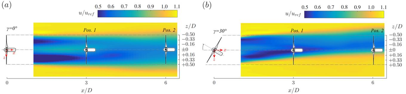
**Figure 2.** Topview of the aligned downstream turbine operated in the wake of an upstream turbine at the two different positions  $x/D = 3$  and  $x/D = 6$ . The wake flow is indicated by measured example cases for **(a)**  $\gamma_{T1} = 0^\circ$  and **(b)**  $\gamma_{T1} = 30^\circ$ .
