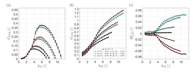
Figure 7. Downstream turbine (a) power coefficient, (b) thrust coefficient and (c) normalized yaw moment as a function of its tip speed ratio  $\lambda_{T2}$  for different lateral offset positions  $\Delta z/D$ . The upstream turbine yaw angle is kept constant at  $\gamma_{T1} = 0^{\circ}$ . The downstream turbine T2 is located at x/D = 3. The turbines are exposed to inflow B.
