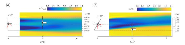
Figure 6. Topview of two lateral offset positions ((a)  $\Delta z/D = -0.16$  and (b)  $\Delta z/D = +0.33$ ) of the downstream turbine while operated in the wake of an upstream turbine at x/D = 3. The upstream turbine is operated at (a)  $\gamma_{T1} = 0^{\circ}$  and (b)  $\gamma_{T1} = 30^{\circ}$ .
