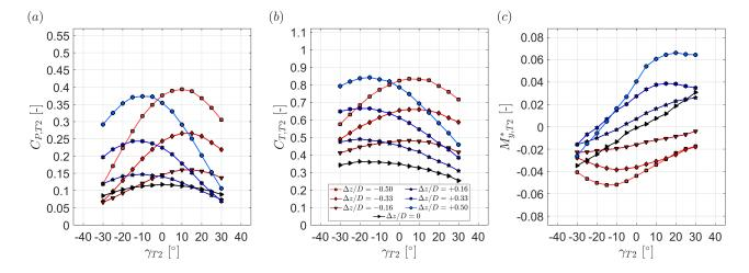
Figure 11. Downstream turbine (a) power coefficient, (b) thrust coefficient and (c) normalized yaw moment as a function of its yaw angle  $\gamma_{T2}$  for different lateral offset positions  $\Delta z/D$ . The upstream turbine yaw angle is kept constant at  $\gamma_{T1}=0^{\circ}$ . The downstream turbine T2 is located at x/D = 3. The turbines are exposed to inflow B.
