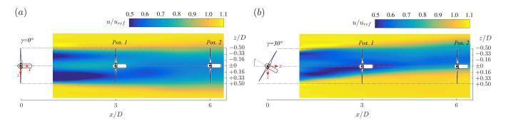
Figure 2. Topview of the aligned downstream turbine operated in the wake of an upstream turbine at the two different positions x/D=3 and x/D=6. The wake flow is indicated by measured example cases for (a)  $\gamma_{T1}=0^{\circ}$  and (b)  $\gamma_{T1}=30^{\circ}$ .
