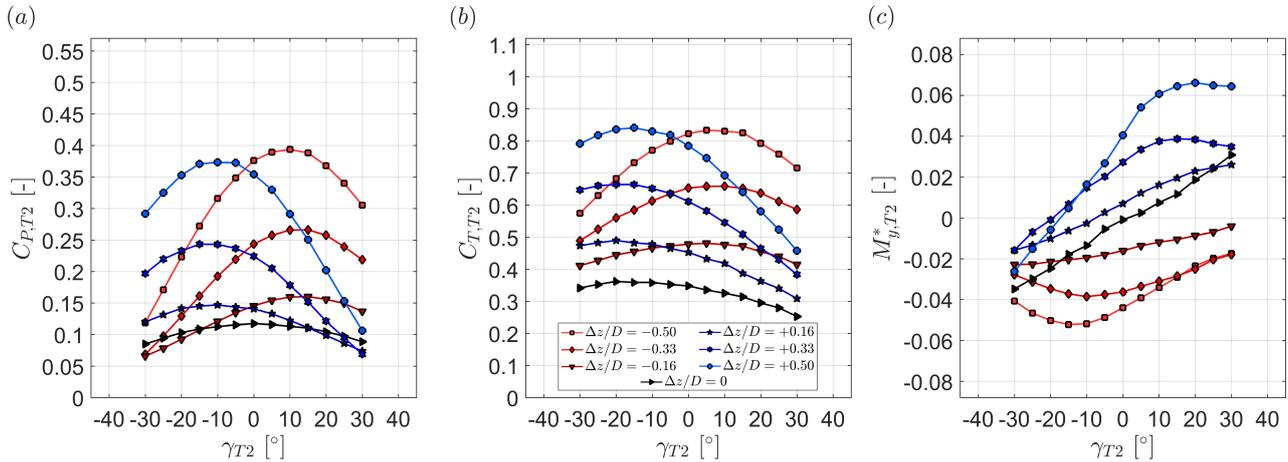
**Figure 11.** Downstream turbine (a) power coefficient, (b) thrust coefficient and (c) normalized yaw moment as a function of its yaw angle  $\gamma_{T2}$  for different lateral offset positions  $\Delta z/D$ . The upstream turbine yaw angle is kept constant at  $\gamma_{T1} = 0^\circ$ . The downstream turbine T2 is located at  $x/D = 3$ . The turbines are exposed to inflow B.
