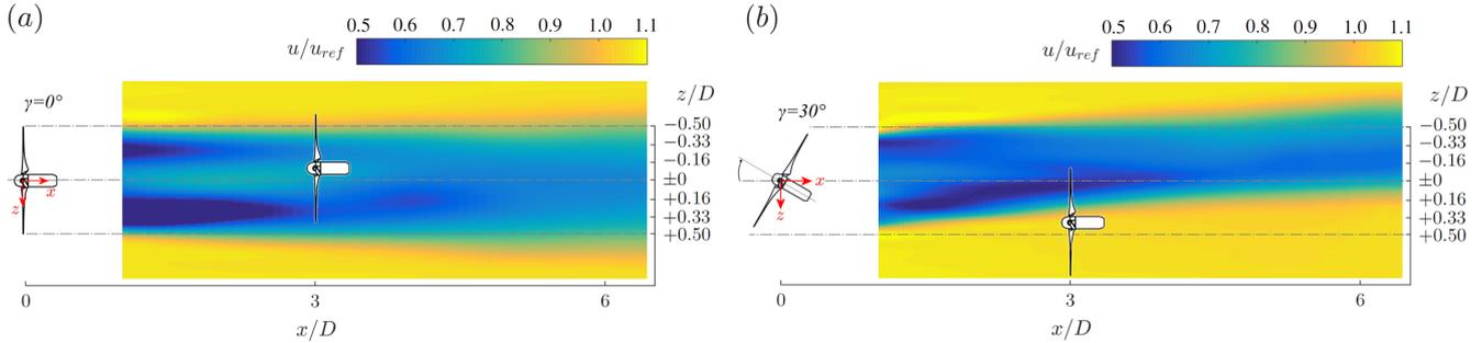
**Figure 6.** Topview of two lateral offset positions ((a)  $\Delta z/D = -0.16$  and (b)  $\Delta z/D = +0.33$ ) of the downstream turbine while operated in the wake of an upstream turbine at  $x/D = 3$ . The upstream turbine is operated at (a)  $\gamma_{T1} = 0^\circ$  and (b)  $\gamma_{T1} = 30^\circ$ .
