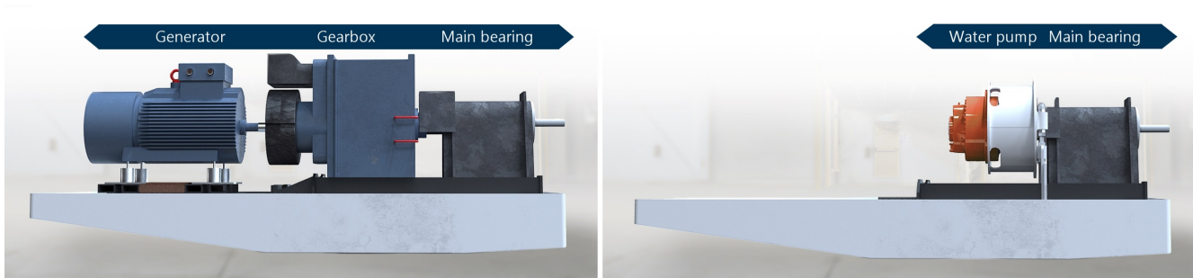
Figure 2. The high power-to-weight ratio of hydraulic components and the possibility to abandon power electronics from the nacelle, make the advantages of mass and space reductions in the nacelle self-evident.
