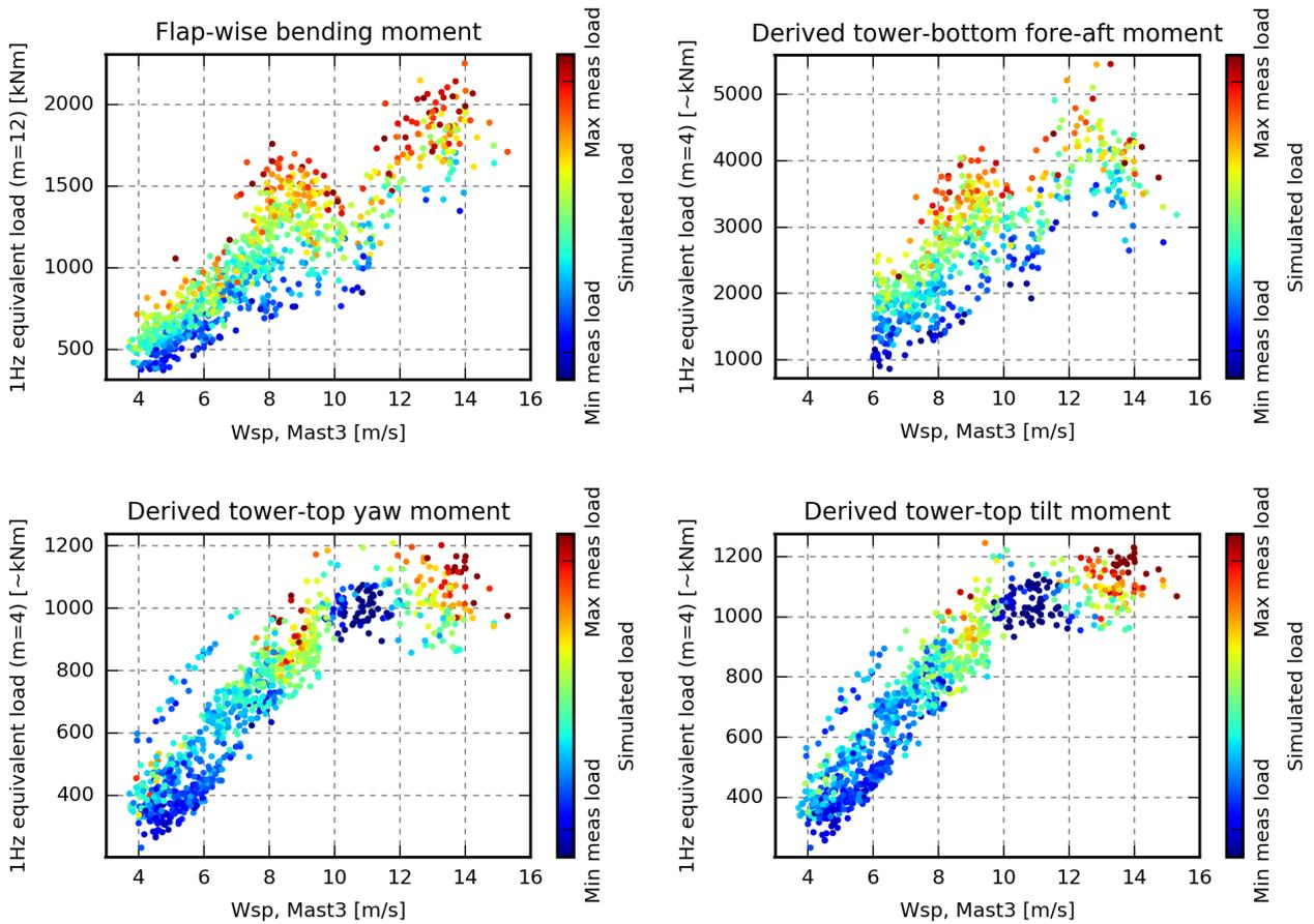
**Figure 18.** Equivalent measured loads, coloured by the corresponding simulation result. The simulations are performed using inflow information from the pitot tube, similar to Case 11 (but only one seed per period). If the simulated load equals the maximum measured load at the current wind speed, then the observation is red, while observations where the simulated load equals the minimum load measured at the current wind speed are blue.
