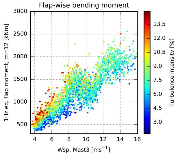
**Figure 2.** The blade-root flap-wise fatigue load plotted as a function of wind speed and coloured by turbulence intensity. The turbulence intensity affects the blade-root fatigue loads. Much of the scatter is, however, caused by other factors.
