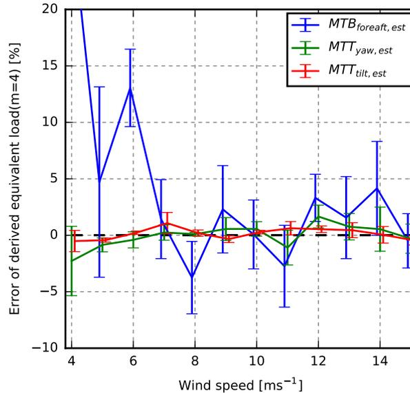
**Figure 5.** Relative fatigue load error of the derived tower load sensors compared to the HAWC2 simulated tower loads. The derived tower load sensors are obtained from the HAWC2 simulated blade-root load sensors and calibrated using wind-speed-dependent calibration constants.
