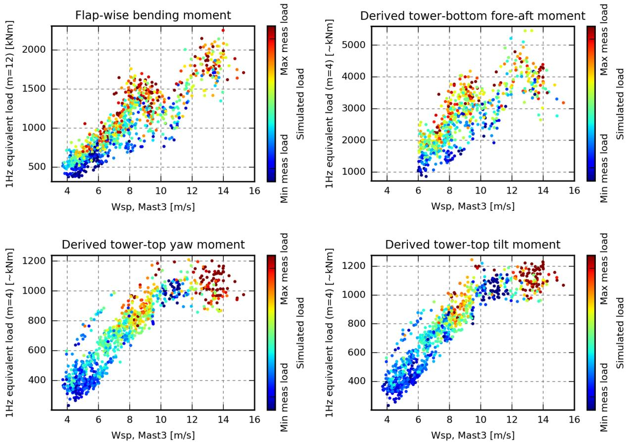
**Figure 17.** Equivalent measured loads, coloured by the corresponding simulation result. The simulations are performed using inflow information from the met masts, similar to **Case 6** (but only one seed per period). If the simulated load equals the maximum measured load at the current wind speed, then the observation is red, while observations where the simulated load equals the minimum load measured at the current wind speed are blue.
