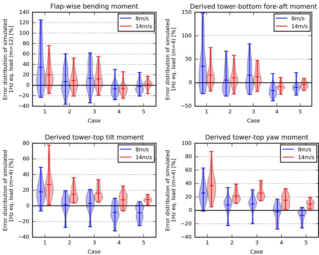
**Figure 11.** Error distribution of the simulated equivalent loads.
