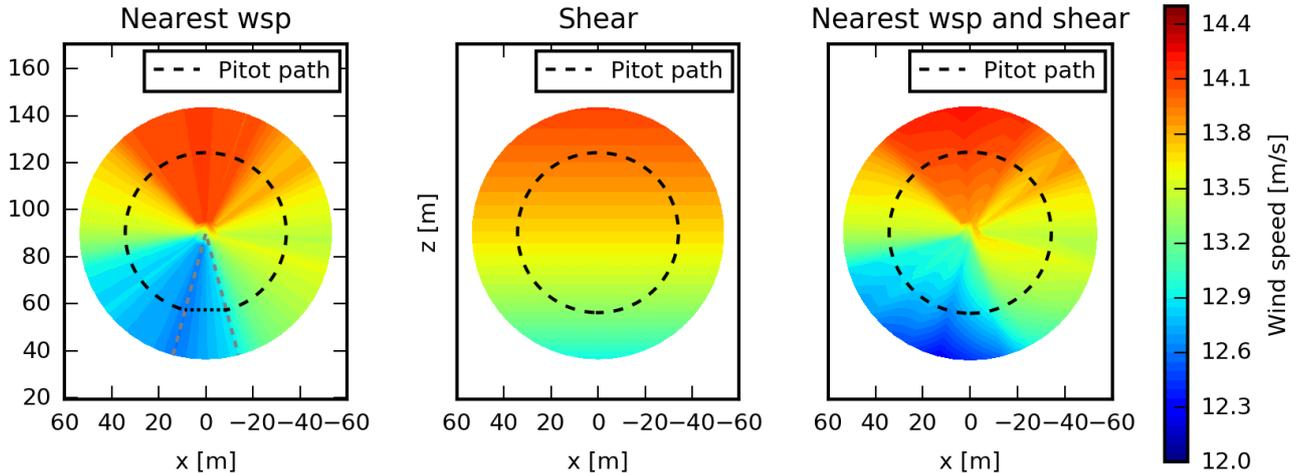
**Figure 6.** Left: wind speed based on nearest pitot-tube wind speed (interpolated values are used in a  $30^\circ$  sector around the tower to the exclude effects of tower shadow). Middle: wind speed based on the one-hour power-shear profile. Right: wind speed based on the nearest pitot-tube wind speed and power shear profile.
