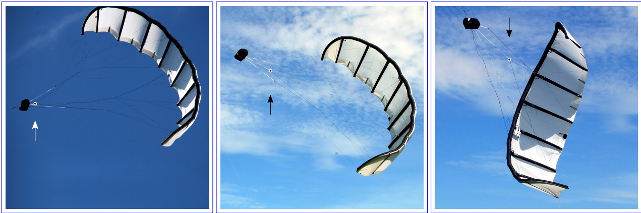
Figure 4. Almost fully powered LEI V3 kite (left), depowered kite (center) and deformation of the wing by extreme steering input in depowered state (right). Dots indicate the end of the depower tape.
