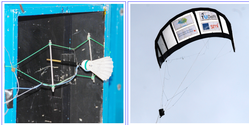
Figure 1. Pitot tube during calibration in the wind tunnel (left) and suspended in the bridle line system of a remote-controlled 25 m 2 LEI V2 kite during a flight test (right).
