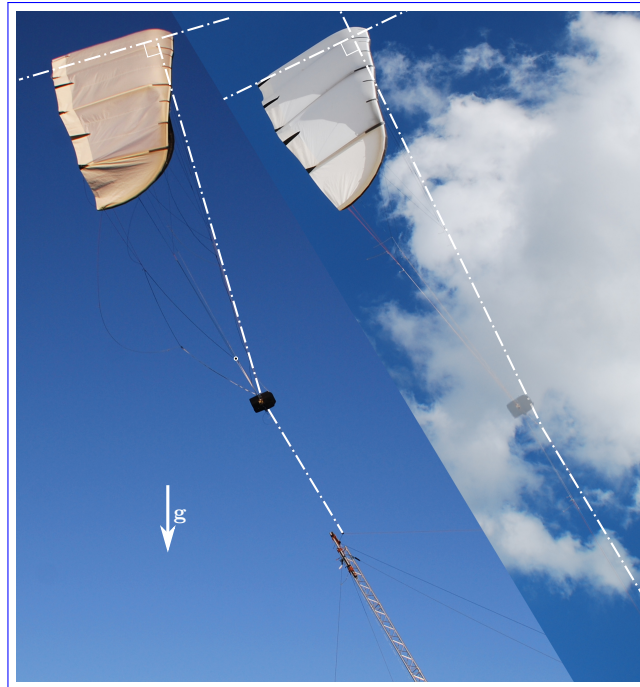
Figure 8. Sideview of kite, partially depowered during landing maneuver (left) and fully powered during crosswind flight maneuver (right). The photo on the right was taken during a flight test in which the KCU was replaced by a ring that collected the joined power lines and the two steering lines and redirect them as a triplet of parallel lines to the pilot on the ground. The position of this ring is hinted by an overlaid transparent image of the KCU.
