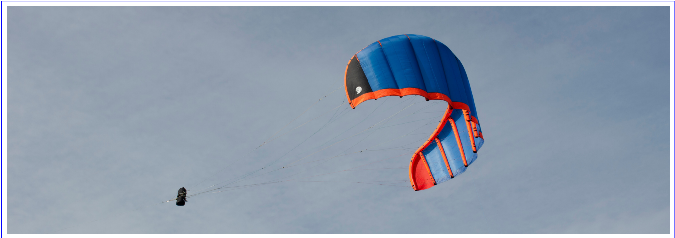
Figure 2. LEI V5.40 kite with 40 m 2 wing surface area controlled by a suspended cable robot. This prototype temporarily reached a tether force of 15 kN and a mechanical power of 100 kW during a test flight in May 2018 (Kitepower B.V., 2018).
