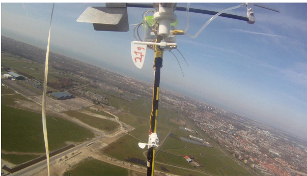
Figure 10. Photo of the in situ measurement setup (left), diagram showing raw values of apparent flow velocity v_a and inflow angles over time during an exemplary traction phase (right).
