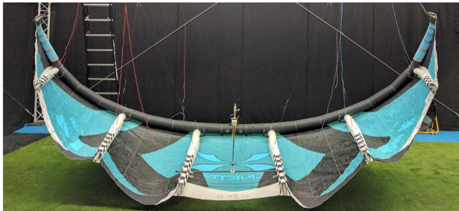
Fig. 1. Center chord parallel air data boom as it was used in [Oehler, J., van Reijen, M., and Schmehl, R.: Experimental investigation of soft kite performance during turning maneuvers]
