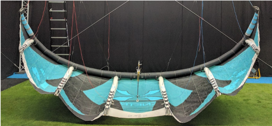
Fig. 1. Center chord parallel air data boom as it was used in [Oehler, J., van Reijen, M., and Schmehl, R.: Experimental investigation of soft kite performance during turning maneuvers]
