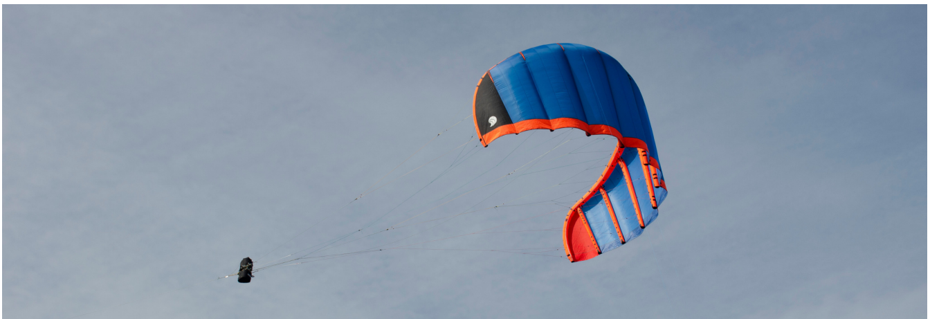
Figure 2. LEI V5.40 kite with 40 \text{ m}^2 wing surface area controlled by a suspended cable robot. This prototype temporarily reached a tether force of 15 kN and a mechanical power of 100 kW during a test flight in May 2018 (Kitepower B.V., 2018).
