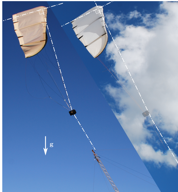
Figure 8. Sideview of kite, partially depowered during landing maneuver (left) and fully powered during crosswind flight maneuver (right). The photo on the right was taken during a flight test in which the KCU was replaced by a ring that collected the joined power lines and the two steering lines and redirect them as a triplet of parallel lines to the pilot on the ground. The position of this ring is hinted by an overlaid transparent image of the KCU.
