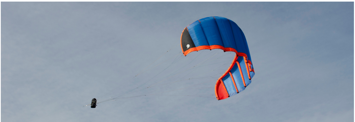
Figure 2. LEI V5.40 kite with 40 \text{ m}^2 wing surface area controlled by a suspended cable robot. This prototype temporarily reached a tether force of 15 kN and a mechanical power of 100 kW during a test flight in May 2018 (Kitepower, 2018).
