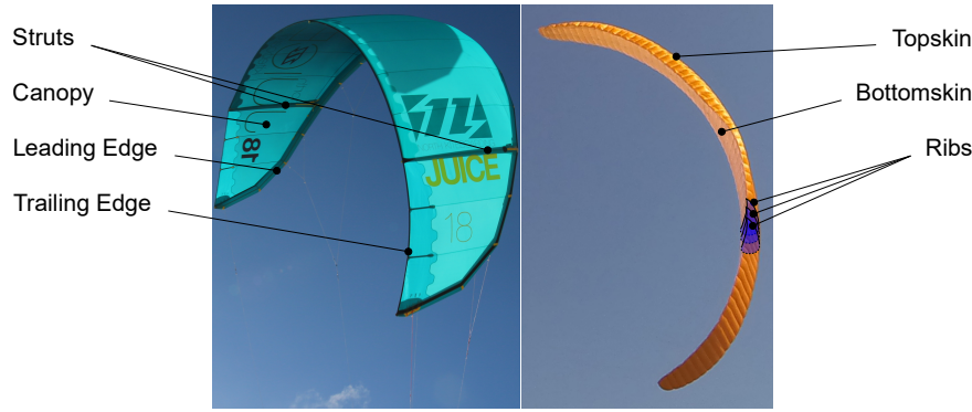
Figure 1. left: Leading Edge Inflatable (LEI) tube kites (single-skin kite); right: ram air wing
