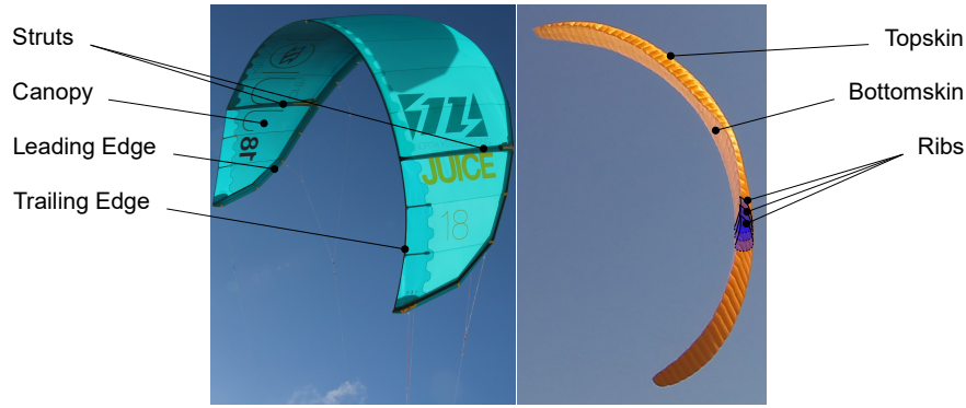
Figure 1. left: Leading Edge Inflatable (LEI) tube kite (single-skin kite); right: ram air wing
