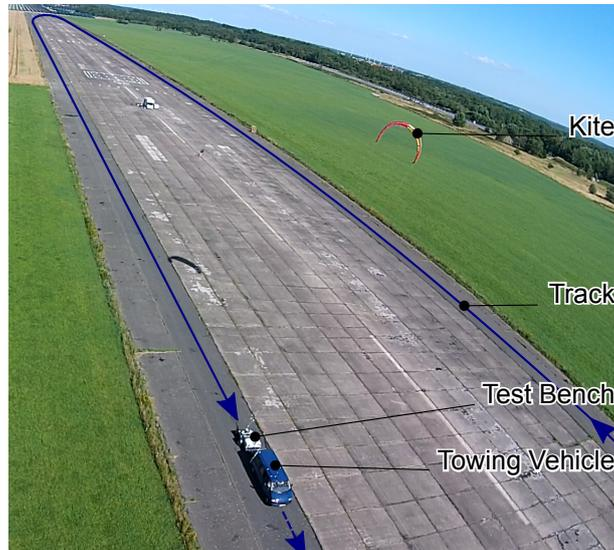
**Figure 11.** Dynamic test procedure
