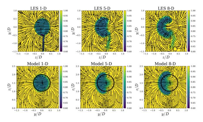
**Figure 2.** Comparison of streamwise velocity contours between a large-eddy simulation (LES) using an actuator disk model without rotation under uniform inflow from Howland et al. (2016) (top) and the proposed model (bottom). The streamlines show the spanwise velocity components.
