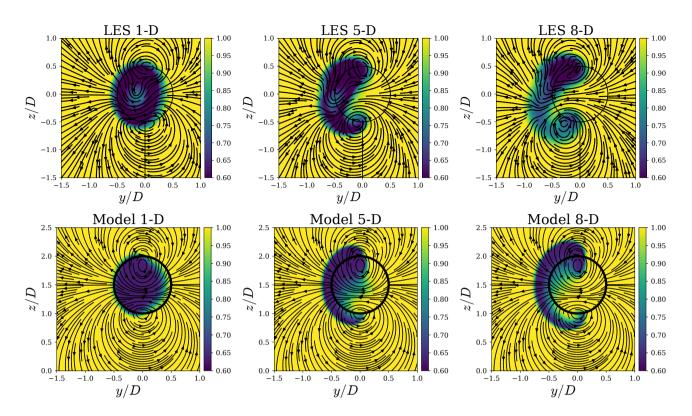
**Figure 3.** Comparison of streamwise velocity contours between a large-eddy simulation using an actuator line model under uniform inflow from Howland et al. (2016) (top) and the proposed model (bottom). The streamlines show the spanwise velocity components.
