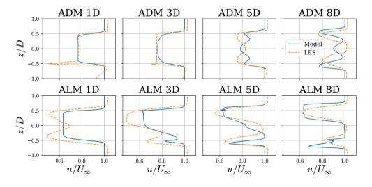
**Figure 5.** Comparison of axial velocity along a vertical line passing through the center of the rotor between a large-eddy simulation using an actuator disk model (top) and actuator line model (bottom) under uniform inflow from Howland et al. (2016) and the proposed model.
