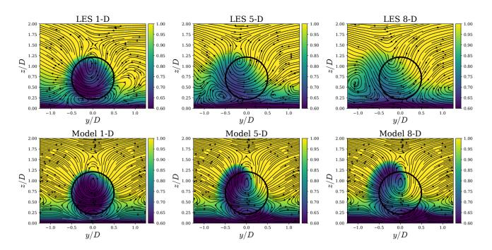
**Figure 7.** Comparison of streamwise velocity contours for the proposed model (bottom) with large-eddy simulations of a wind turbine inside the atmospheric boundary layer (top). The streamlines show the spanwise velocity components.
