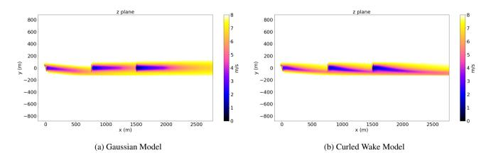
Figure 11. FLORIS simulation of three aligned wind turbines yawing the first turbine 25°.
