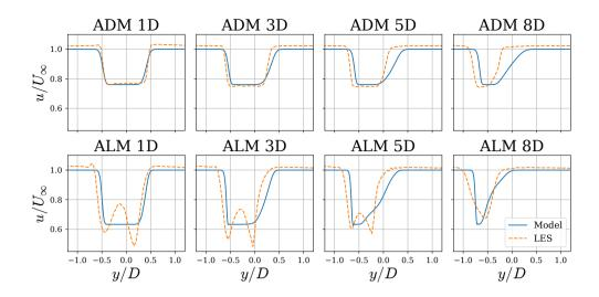
**Figure 4.** Comparison of axial velocity along a horizontal line between a large-eddy simulation using an actuator disk model (top) and actuator line model (bottom) under uniform inflow from Howland et al. (2016) and the proposed model.
