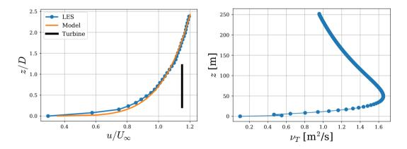
Figure 6. Atmospheric boundary layer inflow (left) from the LES and from a power law used in the model with shear exponent  $\alpha = 0.15$ . The corresponding turbulence viscosity profile (right) as a function of height is shown.
