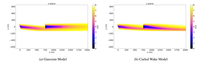
**Figure 10.** FLORIS simulation of two aligned wind turbines yawing the first turbine 25°.
