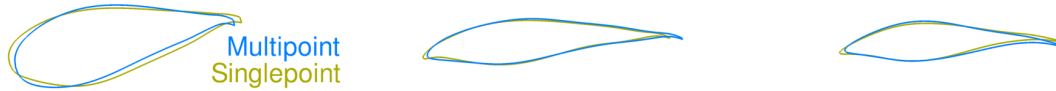
Figure 23. Comparison of profiles obtained from singlepoint and multipoint optimizations. The single point slices are from 35 m, 64 m, and 84 m span and are also seen in Fig. 20.
