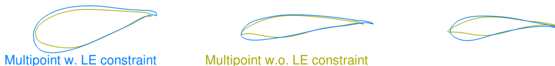
Figure 24. Comparison of profiles obtained from multipoint optimizations with (blue) and without (yellow) a geometrical constraint that prevents a collapse of the LE. Comparing the present figure with Fig. 23 it is clear that the geometrical constraint inclusion results in a much rounder LE.
