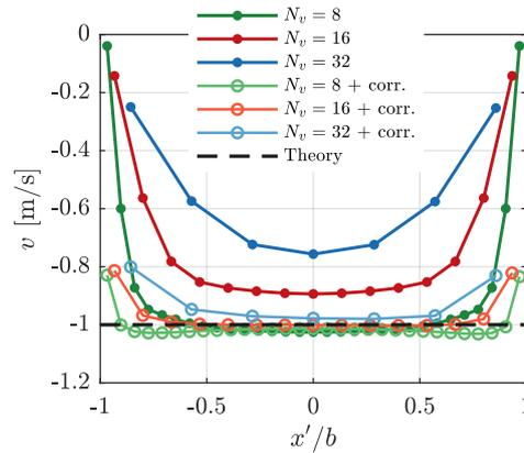
**Figure 8.** Downwash at an elliptical wing predicted by AL simulations with different smearing factors and smearing correction. The CFD component of the velocities are shown (dashed) as well as the total downwash incorporating the correction (solid). The theoretical value acts as reference.
