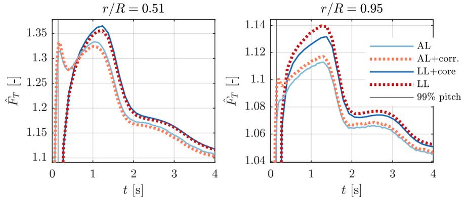
**Figure 14.** Normalised tangential force response at two blade sections (middle and tip) of the NREL 5MW following a pitch step of  $+2^\circ$  in 0.14 s at  $14 \text{ ms}^{-1}$  predicted by AL simulations with/without smearing correction and LL with/without viscous core. ( $N_s = 9$ ,  $\epsilon = 0.2R$ )
