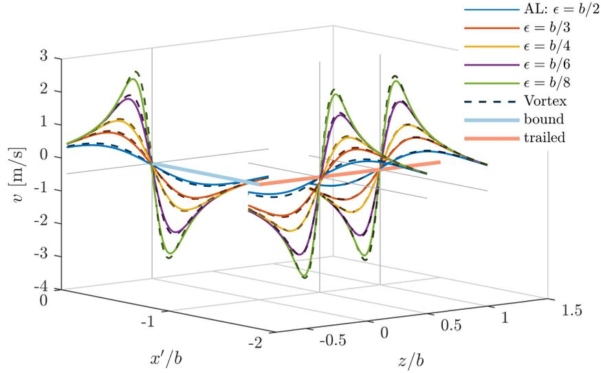
**Figure 6.** Velocities induced perpendicular to a rectangular wing predicted by an actuator line (AL) without correction and by vortex segments with a viscous core (Vortex) with different smearing parameters. Velocities are shown along lines cutting the bound and trailed vortices at right angles and  $y = 0$ . Only half of the horseshoe vortex is depicted as  $x' = x - (b + r_{v=1})$ .
