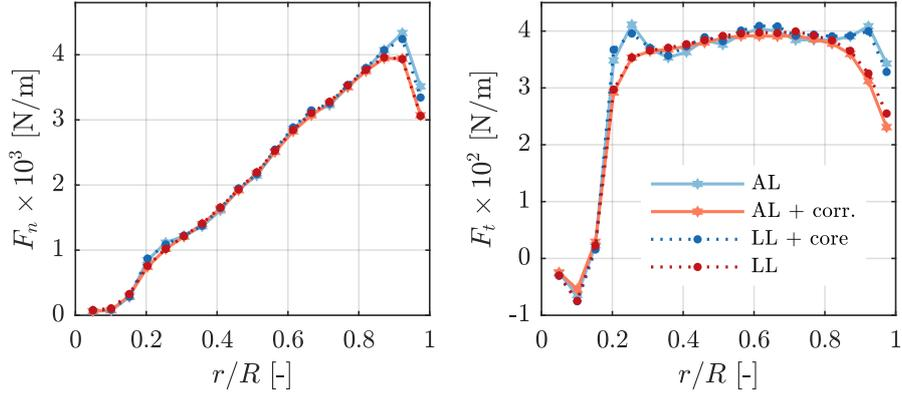
**Figure 9.** Normal and tangential forces on the NREL 5MW blades at  $8 \text{ ms}^{-1}$  predicted by AL simulations with/without smearing correction and LL with/without viscous core. ( $N_s = 19$ ,  $\epsilon = 0.1R$ )
