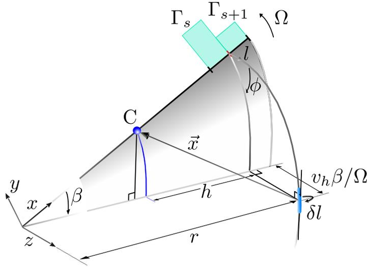
**Figure 4.** Trailed vorticity path. The blade rotates in the  $x$ - $y$  plane and  $z$  points downstream. The vortex element  $\delta l$  with strength  $\Gamma_s - \Gamma_{s+1}$  is shed at  $r$  and transported downstream by the local velocity. The distance from the shedding location  $r$  to a point  $C$  along the blade is  $h$  ( $h = r - C_x$ ), where  $\delta l$  induces tangential and axial velocities.
