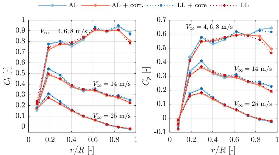
**Figure 12.** Local thrust and power coefficients along the NREL 5MW blades at different wind speeds predicted by AL simulations with/without smearing correction and LL with/without core. ( $N_s = 9$ ,  $\epsilon = 0.2R$ )
