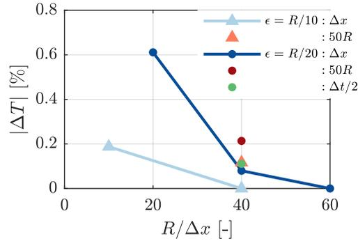
**Figure 3.** Thrust sensitivity of the NREL 5MW AL simulations at  $8 \text{ ms}^{-1}$  wind speed with grid size, doubling the domain size and halving the time step at two smearing length scales. ( $N_s = \{9, 19\}$ ,  $T_{\text{ref}} = \{4.20, 4.06\} \times 10^5$  N)
