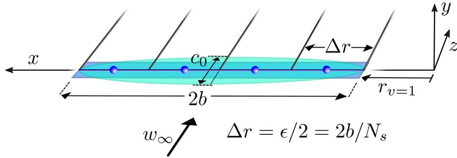
**Figure 5.** Definition of the wing test cases with either a rectangular or elliptic planform. Vortices are trailed in-between sections and the actuator line forces are computed and exerted at the sections' centres.
