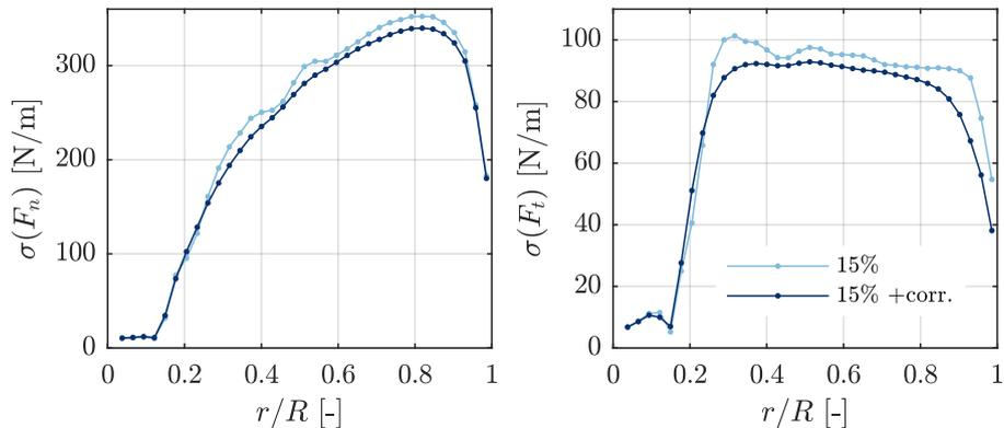
**Figure 16.** Variation of normal and tangential forces on the NREL 5MW blades at  $8 \text{ ms}^{-1}$  mean wind speed and turbulence intensity of 15% predicted by the AL model with and without smearing correction. ( $N_s = 35$ ,  $\epsilon = R/8$ )
