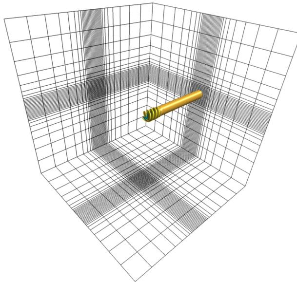
**Figure 2.** Numerical box domain with a structured mesh and uniform spacing around the rotor at its centre. Only every eighth grid point and half of the domain is shown.
