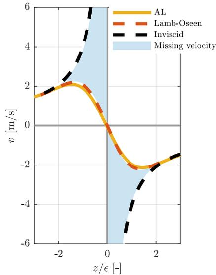
**Figure 1.** Distribution of the tangential velocity component in a plane orthogonal to an infinite vortex line (along  $x$ ) obtained from either an inviscid or viscous (Lamb-Oseen) theoretical vortex and an actuator line CFD simulation.
