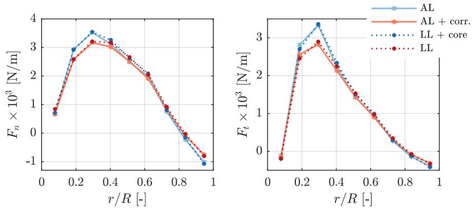
**Figure 11.** Normal and tangential forces on the NREL 5MW blades at  $25 \text{ ms}^{-1}$  predicted by AL simulations with/without smearing correction and LL with/without viscous core. ( $N_s = 9$ ,  $\epsilon = 0.2R$ )
