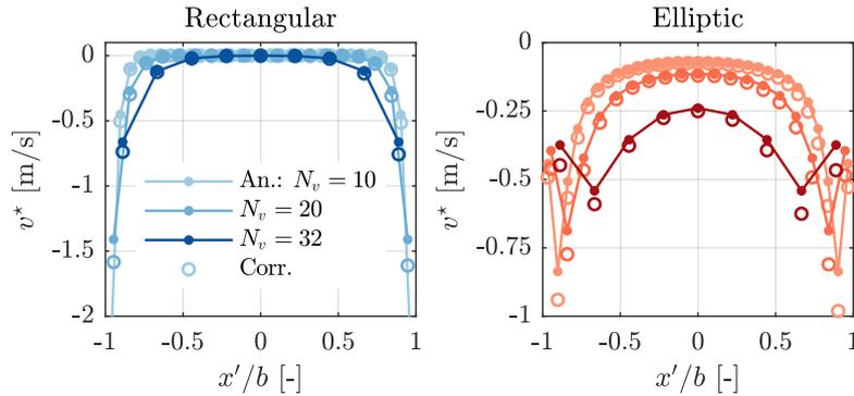
**Figure 7.** Analytical (An.) and corresponding model prediction of the velocity correction for varying force smearing ( $\epsilon = 2b/(N_v - 1)$ ) along a rectangular and elliptic wing, where  $x' = x - (b + r_{v=1})$ .
