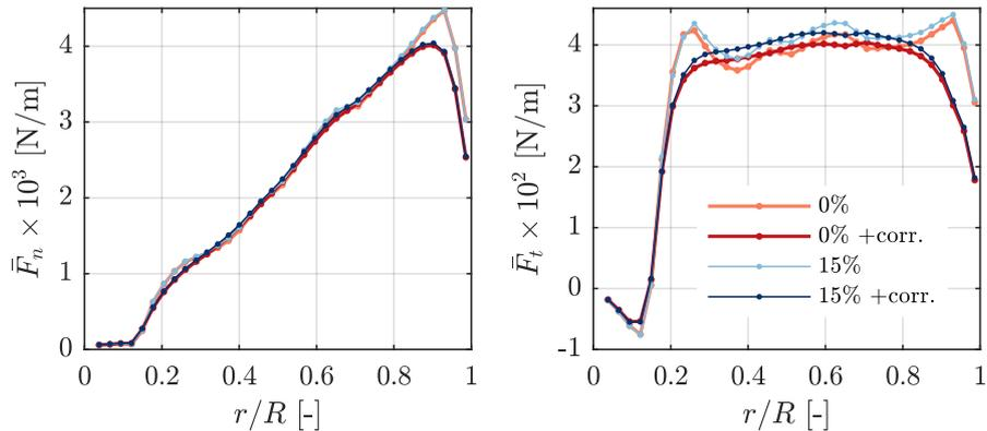
**Figure 15.** Time-averaged normal and tangential forces on the NREL 5MW blades at  $8 \text{ ms}^{-1}$  mean wind speed and changing inflow turbulence predicted by the AL model with and without smearing correction. ( $N_s = 35$ ,  $\epsilon = R/8$ )
