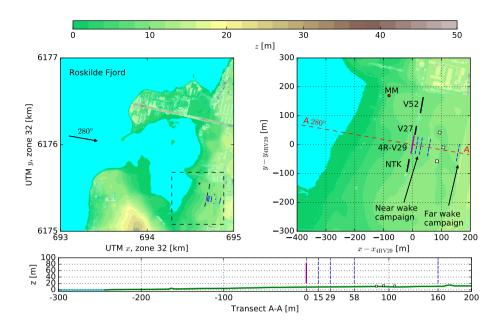
**Figure 5.** Topography around the 4R-V29 wind turbine and overview of wake measurements. Right top plot is a zoom of the left top plot. Bottom plot is the terrain height along transect A-A. Location of three WindScanners are shown as white squares, scanning locations are shown as blue dashed lines, MM is the met mast, and V52, V29 and NTK are neighboring wind turbines.
