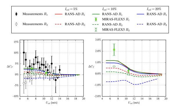
**Figure 11.** Rotor individual relative difference between the 4R-V29 wind turbine with all rotors in operation and the 4R-V29 wind turbine with a single rotor in operation, in terms of power and thrust as function of the freestream velocity at a height of 44.27 m.
