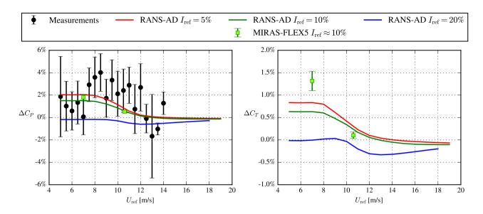
**Figure 10.** Relative difference between the 4R-V29 wind turbine with all rotors in operation and the 4R-V29 wind turbine with a single rotor in operation, in terms power and thrust as function of the freestream velocity at a height of 44.27 m.
