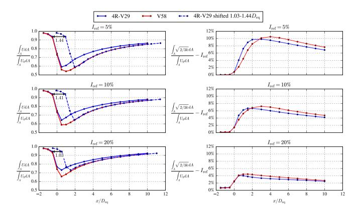
**Figure 18.** RANS predicted wake recovery of a simplified 4R-V29 multi-rotor wind turbine compared with an equivalent V58 single-rotor wind turbine for three difference turbulence intensities. Left plot: integrated stream-wise velocity, right plot: integrated added turbulence intensity. Dashed blue line is the integrated stream-wise velocity of the simplified 4R-V29 wind turbine shifted by 1.03-1.44*D*.
