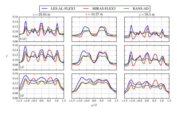
Figure 14. Near wake case: Profiles of turbulence intensity at three heights and three downstream distances.
