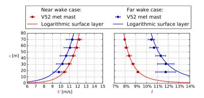
Figure 7. Profiles of wind speed and turbulence intensity measured at the met mast and corresponding logarithmic surface layer using  $U_{\text{ref}}$  and  $I_{\text{ref}}$  from Tab. 1 for the near and far wake measurement cases. Error bars represent the standard error of the mean.
