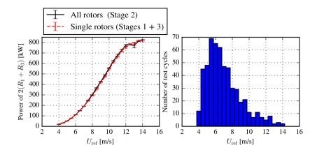
**Figure 4.** Left: Measured electric power of  $2(R_1 + R_3)$  from the 4R-V29 wind turbine as function of the freestream velocity at a height of 44.27 m for all rotors and single rotors in operation. Error bars represents the standard error of the mean power. Right: Number of test cycles.
