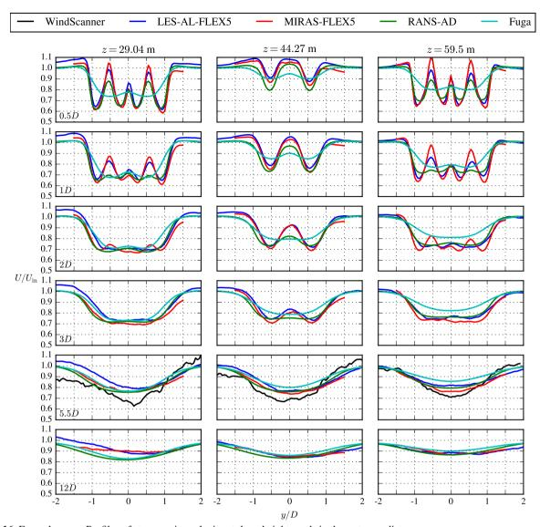
Figure 16. Far wake case: Profiles of stream-wise velocity at three heights and six downstream distances.
