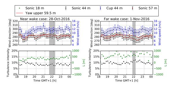
**Figure 6.** Atmospheric conditions during the near and far wake measurements as measured at V52 met mast. Top plots: Wind direction and wind speed and yaw angle of the upper platform. Bottom plots: Total turbulence intensity and Monin Obukhov length. Error bars represent the standard error of the mean. Gray area depict the time of the chosen measurements.
