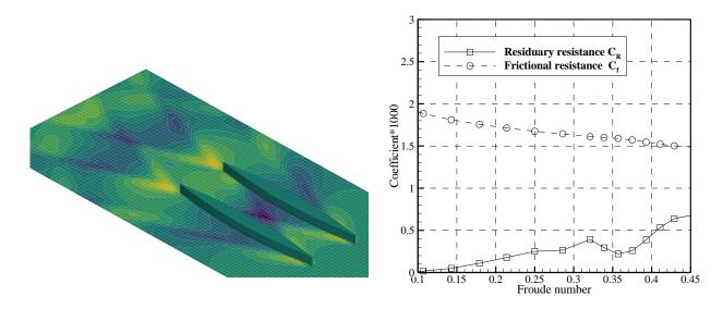
Figure 10 Picture of the hull shape considered in this study and related hydrodynamic coefficients
