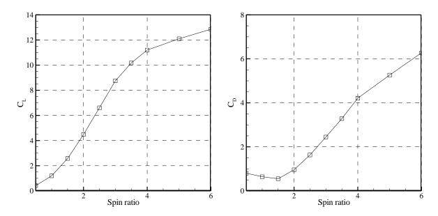
Figure 8 Experimental results of Charrier (Charrier, 1979) for the aerodynamic coefficients of a Flettner rotor. Left figure is the lift coefficient. The right figure shows the drag coefficient. In the experiments, the rotor was fitted with end discs at both ends. The diameter of the discs was twice the diameter of the rotor. The aspect ratio of the rotor was 5 and the Reynolds number was 13,200.
