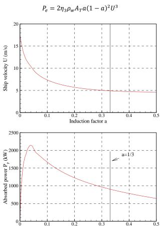
Figure 4 Ship velocity (top) and absorbed power (bottom) as function of the induction factor. The true wind speed is 10 m/s and the true wind angle is 90°. The wind propulsion subsystems are Flettner rotors. The spin ratio is 3. Constraints on maximum rotational velocity, maximal thrust and cut-out speed are not taken into account in this example.
