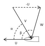
Figure 3 Definitions of the true wind angle  $\beta$  and apparent wind angle  $\alpha$ .
