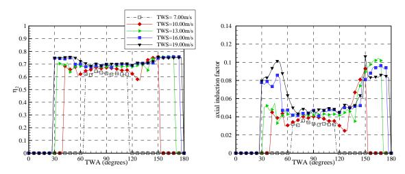
Figure 12 Efficiency of the conversion of wind energy into mechanical energy by the proposed energy ship design (left) and optimal induction factor (right) as function of the wind conditions. TWS stands for true wind speed.
