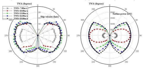
Figure 11 Velocity (left) and generated power (right) polar plots of the proposed energy ship design for true wind speeds of 7, 10, 13, 16 and 19 m/s. TWA stands for true wind angle.
