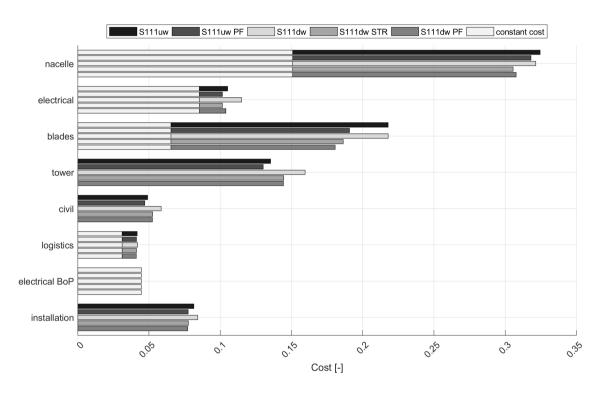
**Figure 6.** Turbine CAPEX cost split by main cost components normalized by the sum of the S111uw configuration with indication of constant costs not affected by redesign process.
