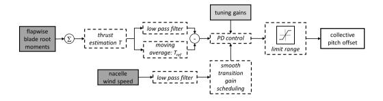
**Figure 2.** Flow chart of the thrust control controller addition.
