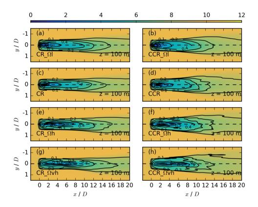
**Figure 14.** Contours of the streamwise velocity  $\overline{u_{i,j,k_*}}$  in m s<sup>-1</sup> for different rotational frequencies at z = 100 m for CR\_ $\Omega$ l in (a), CCR\_ $\Omega$ l in (b), CR in (c), CCR in (d), CR\_ $\Omega$ h in (e), CCR\_ $\Omega$ h in (f), CR\_ $\Omega$ vh in (g), and CCR\_ $\Omega$ vh in (h), each averaged over 30 min. The black contours represent the velocity deficit  $VD_{i,j,k_*}$  at the same vertical location.
