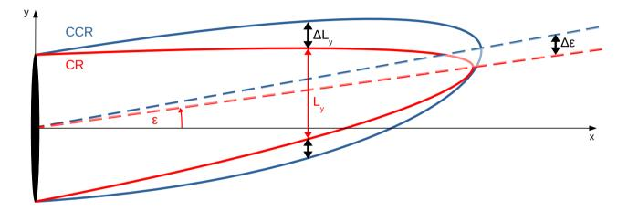
**Figure 20.** Schematic illustration of the difference in the spanwise wake width  $(L_y)$  and the wake deflection angle  $(\epsilon)$  between clockwise CR and counterclockwise CCR rotating actuators. The parameter impact on the these wake differences is represented by  $\Delta L_y$  and  $\Delta \epsilon$ .
