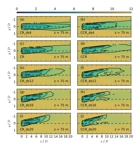
**Figure 12.** Contours of the streamwise velocity  $\overline{u_{i,j,k_*}}$  in m s<sup>-1</sup> for different directional shears at z = 75 m for the same simulations as in Fig. 10. The black contours represent the velocity deficit  $VD_{i,j,k_*}$  at the same vertical location.
