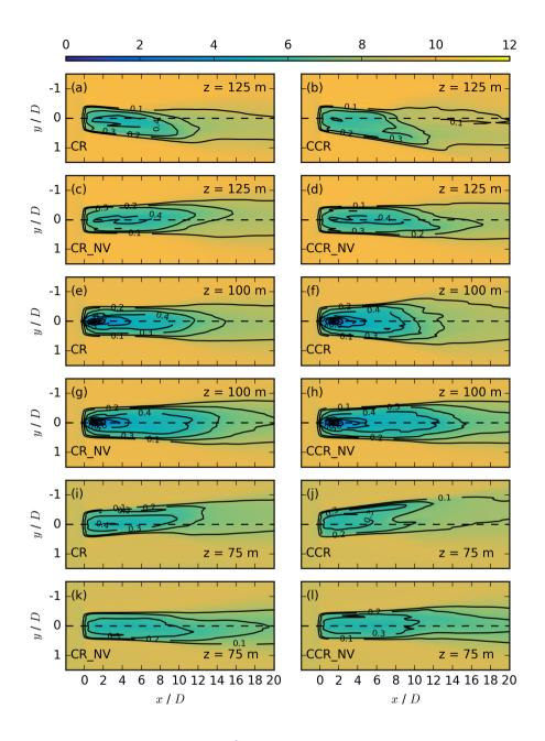
**Figure 4.** Contours of the streamwise velocity  $\overline{u_{i,j,k_*}}$  in m s<sup>-1</sup> at z = 125 m in the first two rows, at z = 100 m the the third and fourth row, and at z = 75 m in the last two rows for the simulations CR, CCR, CR\_NV and CCR\_NV, each averaged over 30 min. The black contours represent the velocity deficit  $VD_{i,j,k_*}$  at the same vertical location.
