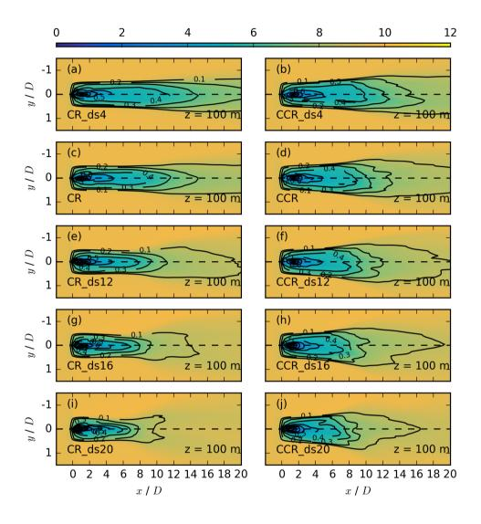
**Figure 10.** Contours of the streamwise velocity  $\overline{u_{i,j,k_{s}}}$  in m s<sup>-1</sup> for different directional shears at z = 100 m for CR\_ds4 in (a), CCR\_ds4 in (b), CR in (c), CCR in (d), CR\_ds12 in (e), CCR\_ds12 in (f), CR\_ds16 in (g), CCR\_ds16 in (h), CR\_ds20 in (i), and CCR\_ds20 in (j), each averaged over 30 min. The black contours represent the velocity deficit  $VD_{i,j,k_{s}}$  at the same vertical location.
