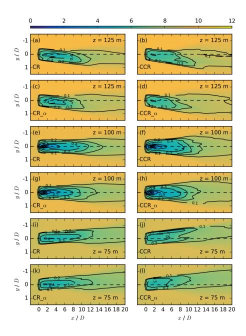
**Figure A1.** Contours of the streamwise velocity  $\overline{u_{i,j,k_*}}$  in m s<sup>-1</sup> at z = 125 m in the first two rows, at z = 100 m the the third and fourth row, and at z = 75 m in the last two rows for the simulations CR, CCR, CR\_ $\alpha$  and CCR\_ $\alpha$ , each averaged over 30 min. The black contours represent the velocity deficit  $VD_{i,j,k_*}$  at the same vertical location.
