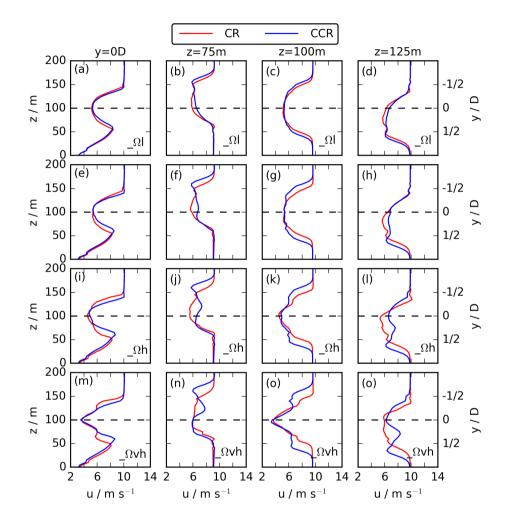
Figure 17. Vertical (first column) and horizontal profiles at z = 75 m (second column), z = 100 m (third column), and z = 125 m (fourth column) of the 30 min averaged streamwise velocity at x = 7 D downwind of the actuator for a rotational frequency of  $\Omega = 0.058^{\circ}$  s<sup>-1</sup> in (a)-(d),  $\Omega = 0.12^{\circ}$  s<sup>-1</sup> in (e)-(g),  $\Omega = 0.175^{\circ}$  s<sup>-1</sup> in (i)-(l), and  $\Omega = 0.23^{\circ}$  s<sup>-1</sup> in (m)-(o).
