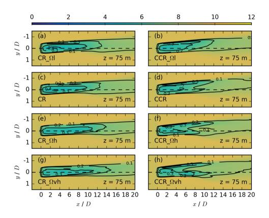
**Figure 16.** Contours of the streamwise velocity  $\overline{u_{i,j,k_*}}$  in m s<sup>-1</sup> for different rotational frequencies at z = 75 m for the same simulations as in Fig. 14. The black contours represent the velocity deficit  $VD_{i,j,k_*}$  at the same vertical location.
