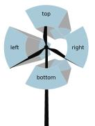
Figure 1. Schematic illustration of the top sector, the bottom sector, as well as the left and right sectors, defined from a view looking downwind towards the wind turbine on the disc.
