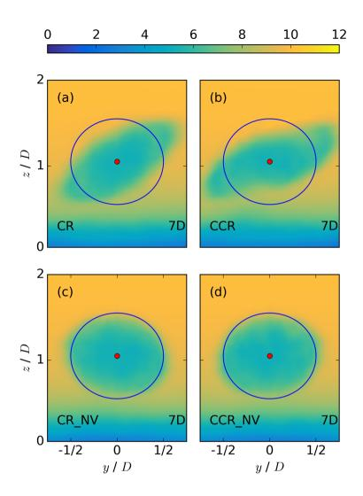
Figure 5. Contours of the streamwise velocity  $\overline{u_{i,j,k_{\pi}}}$  in m s<sup>-1</sup> at a downward position of x = 3D behind the rotor of for CR in (a), CCR in (b), CR\_NV in (c), and CCR\_NV in (d). The blue circle represents the circumference of the actuator disc.
