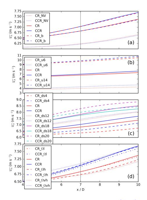
Figure 7. The rotor and time averaged streamwise velocity  $\overline{u_A}$  presented for a downwind region of [4D;10D] with special emphasis at x = 7 D for the simulations CR\_NV, CCR\_NV, CR, CCR, CR\_b and CCR\_b in (a), for different geostrophic wind values in (b), for different directional shears in (c), and for different rotational frequencies in (d).
