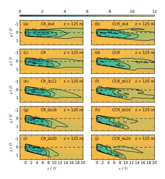
**Figure 11.** Contours of the streamwise velocity  $\overline{u_{i,j,k_*}}$  in m s<sup>-1</sup> for different directional shears at z = 125 m for the same simulations as in Fig. 10. The black contours represent the velocity deficit  $VD_{i,j,k_*}$  at the same vertical location.
