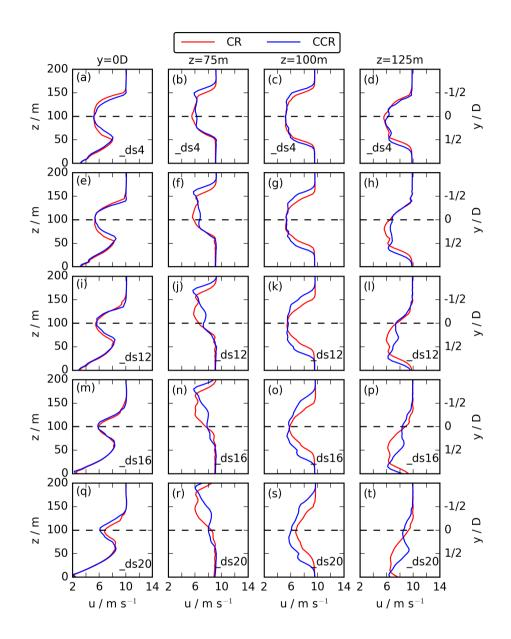
**Figure 13.** Vertical (first column) and horizontal profiles at z = 75 m (second column), z = 100 m (third column), and z = 125 m (fourth column) of the 30 min averaged streamwise velocity at x = 7D downwind of the actuator for a directional shear of  $0.04^{\circ}$  m<sup>-1</sup> in (a)-(d),  $0.08^{\circ}$  m<sup>-1</sup> in (e)-(h),  $0.12^{\circ}$  m<sup>-1</sup> in (i)-(l),  $0.16^{\circ}$  m<sup>-1</sup> in (m)-(p), and  $0.20^{\circ}$  m<sup>-1</sup> in (q)-(t).
