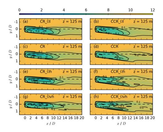
**Figure 15.** Contours of the streamwise velocity  $\overline{u_{i,j,k_*}}$  in m s<sup>-1</sup> for different rotational frequencies at z = 125 m for the same simulations as in Fig. 14. The black contours represent the velocity deficit  $VD_{i,j,k_*}$  at the same vertical location.
