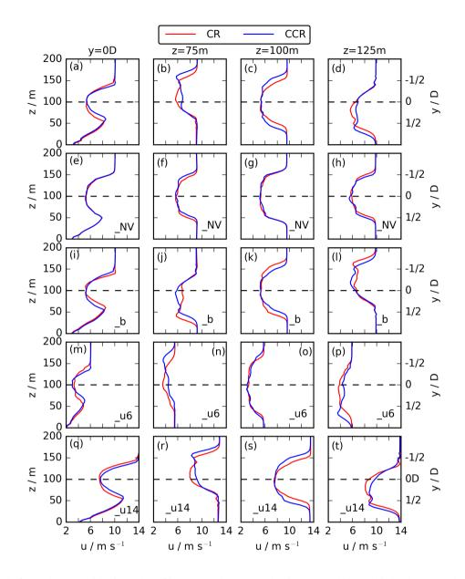
**Figure 6.** Vertical (first column) and horizontal profiles at z = 75 m (second column), z = 100 m (third column), and z = 125 m (fourth column) of the 30 min averaged streamwise velocity at x = 7 D downwind of the actuator for CR and CCR in (a) - (d), CR\_NV and CCR\_NV in (e) - (h), CR\_b and CCR\_b in (i) - (l), CR\_u6 and CCR\_u6 in (m) - (p), and CR\_u14 and CCR\_u14 in (q) - (t).
