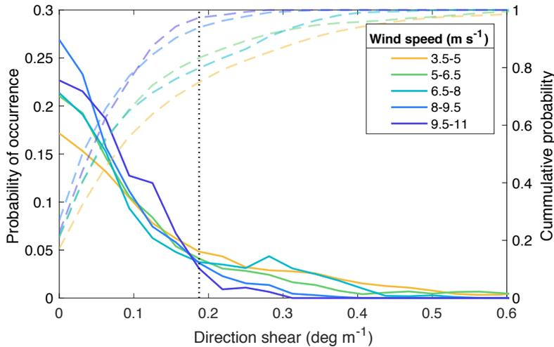
**Figure 11. Directional wind shear probability density (solid lines) and cumulative (dashed lines) distributions for 1.5 m s<sup>-1</sup> wind speed regimes. The black dotted line marks 0.1875 deg m<sup>-1</sup> of directional wind shear.**
