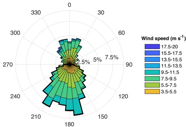
**Figure 3. Wind rose for lidar hub-height altitude (80-m) measured wind speeds between cut-in and cut-out. The black outline highlights the wind direction sector (southerly) used for subsequent data analysis.**
