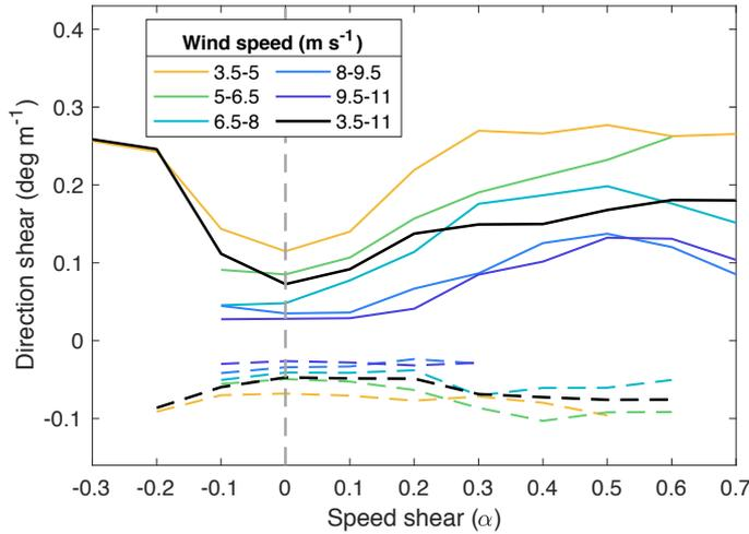
**Figure 13.** Mean speed and direction shear relationship for similar hub-height wind speed regimes ( $1.5 \text{ m s}^{-1}$  bins). Solid lines correspond to wind veering and dashed lines to wind backing. Black lines correspond to the mean for all wind speeds. The dashed grey line marks zero-speed shear value.
