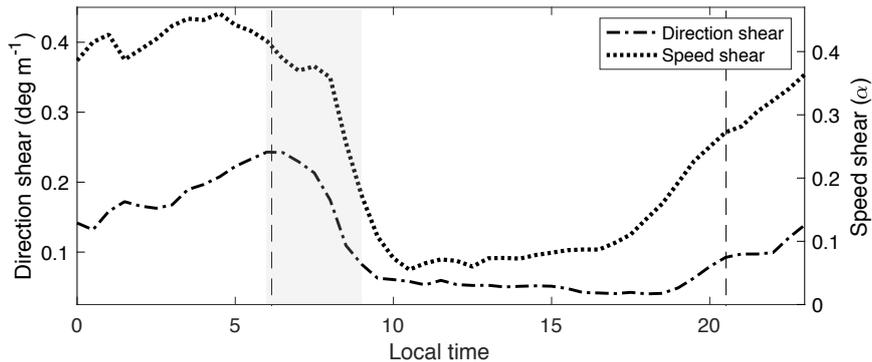
10 **Figure 9. Diurnal cycle of mean wind direction and speed shear for wind speeds between cut-in and cut-out. Dashed vertical lines indicate sunrise and sunset times for August 1, 2013, the mid-point of the dataset analyzed here. The grey shaded region indicates the morning transition period (0600 – 0900 LT).**
