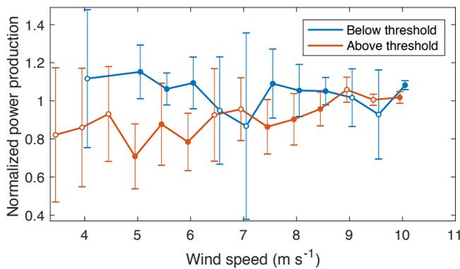
**Figure 16.** Mean normalized power production (turbines A, B, C and D) of observations above and below the  $\alpha/\beta$  threshold for speed shear between 0.3 – 0.4 during the morning transition (0600 – 0900 LT). Filled circles are statistically distinct. Errorbars represent one standard deviation from the mean.
