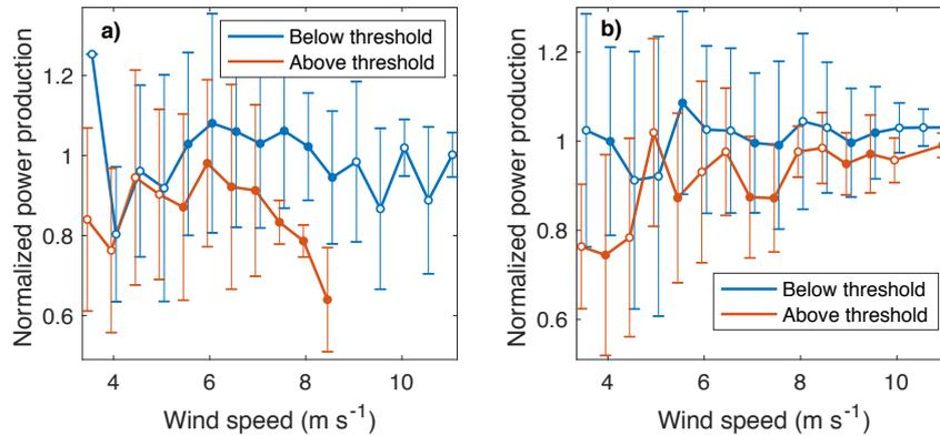
**Figure 15.** Mean normalized power production (turbines A, B, C and D) of observations above and below the  $\alpha/\beta$  threshold for speed shear between 0.2 – 0.3 (a), and 0.4 – 0.5 (b). Filled circles are statistically distinct. Errorbars represent 1 standard deviation from the mean.
