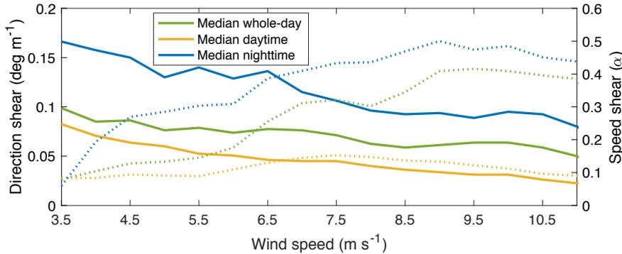
5 **Figure 10. Direction (solid line) and speed (dotted line) wind shear variation with 80-m wind speed using each day’s sunrise/sunset times of day.**
