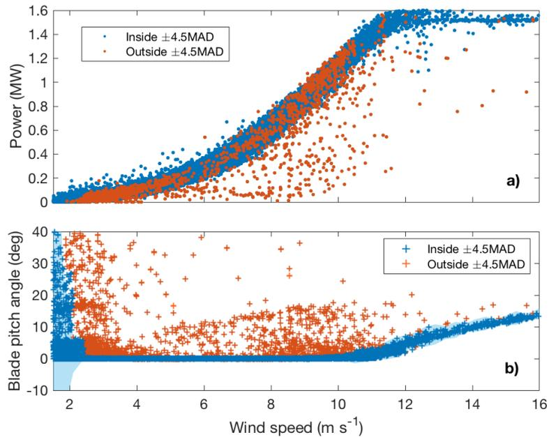
Figure 4. Power curve based on nacelle-measured wind speed (a), and blade pitch angle from a single blade (b) combining data from the four analyzed wind turbines. The blue envelope in the bottom graph represents  $\pm 4.5$  MAD of the blade pitch angle within  $0.5 \text{ m s}^{-1}$  wind speed bins. Red scatter points show 10-min periods filtered out for curtailments, represented by data points outside the MAD envelope.
