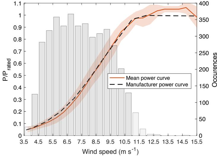
**Figure 6. Mean power curve for Turbine C based on 80-m lidar wind speed measurements overlaid over the number of power production cases for each 0.5 m s<sup>-1</sup> wind speed bins. The shaded region in the power curve corresponds to  $\pm 1$  standard deviation, and the dark grey histogram corresponds to the wind speed ranges considered in this study.**
