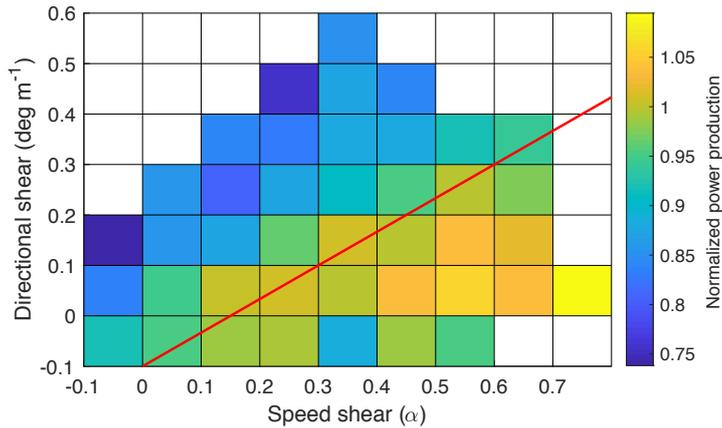
**Figure 14. Mean normalized power production (turbines A, B, C and D) for all combinations of speed and direction shear that present more than 30 observations. The red line represents the  $\alpha/\beta$  threshold.**
