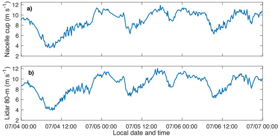
**Figure 5. Time series from 00:00 July 04, 2013 to 00:00 July 07, 2013 of hub-height wind speeds measured by the cup anemometer on the nacelle of Turbine A (a), and 80-m wind speeds measured by the lidar (b).**
