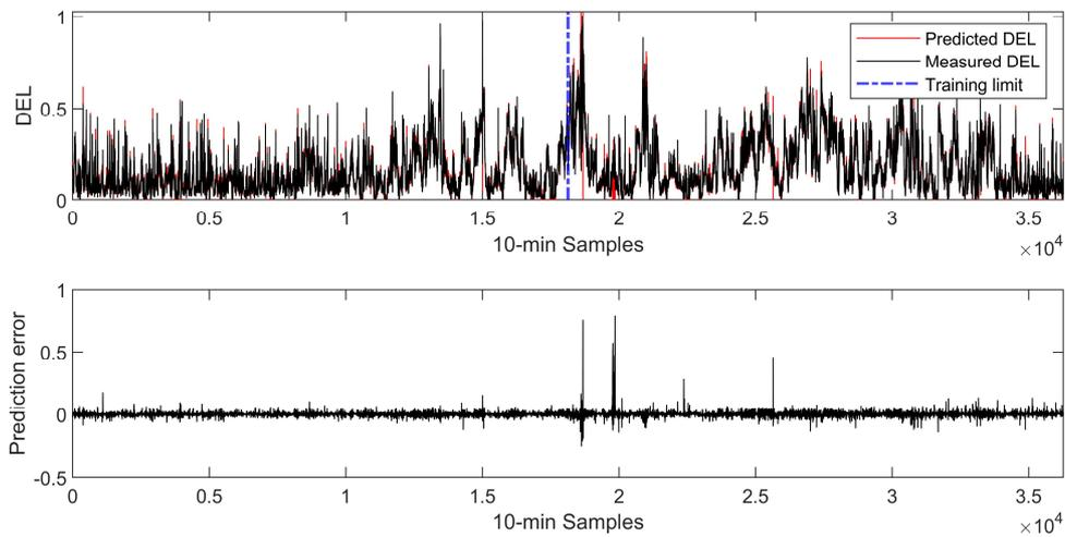
15 **Figure 8 — Comparison of normalized predicted and measured DELs and the corresponding prediction error for the model using the feature-set from the correlation analysis.**
