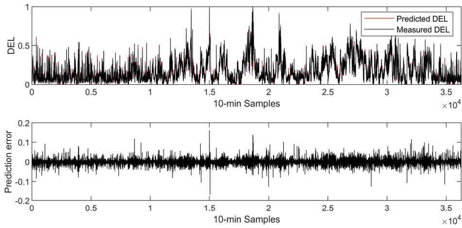
**Figure 5 -- NN prediction: The top plot presents the normalized predicted and the measured DELs by NN. The bottom plot is the prediction error.**
