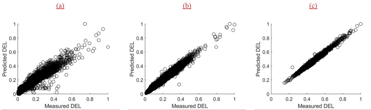
**Figure 7** – Normalized measured vs. predicted DELs. Figures correspond to a model built with features from the correlation analysis. Subfigure (a): Standstill. Subfigure (b): Partial load. Subfigure (c): Full load.
