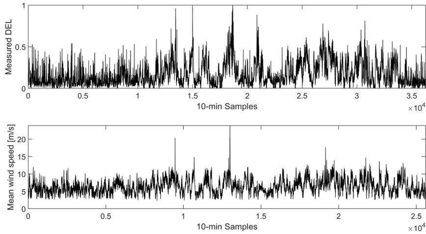
**Figure 2 – Normalized DELs and mean wind speed**
