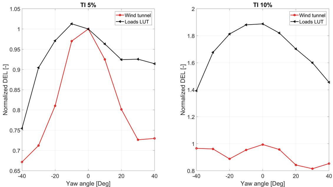
**Figure 5.** CL-Windcon and loads module tower base fore-aft moment as a function of yaw, for low turbulence (left) and high turbulence (right)
