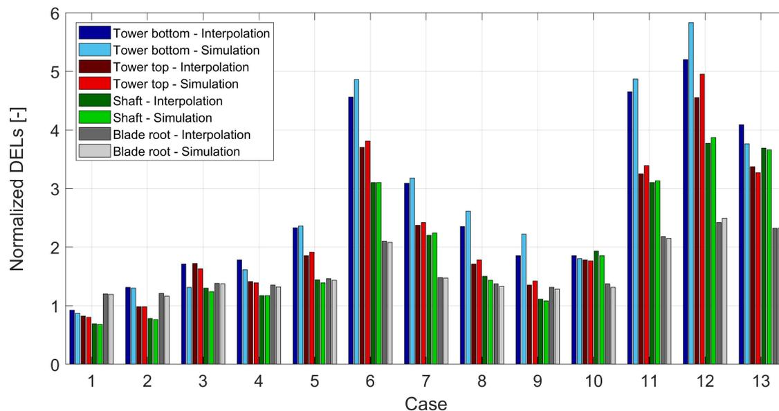
**Figure 2.** Visualization of interpolation and BEM simulation results. When all the parameters are changed at a time, the bigger discrepancies observed for tower at bottom moments
