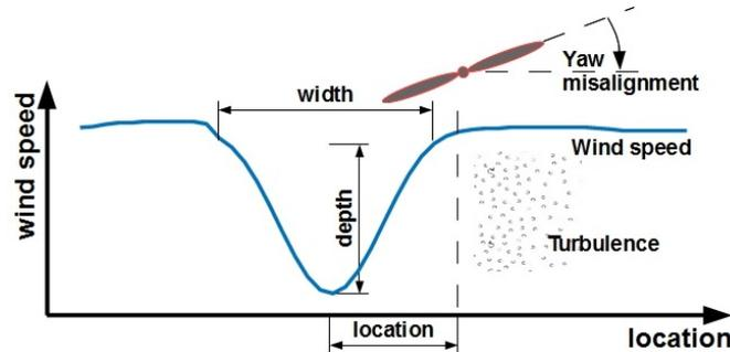
**Figure 1.** Visualization of the parameters used for describing the wake conditions in front of a turbine
