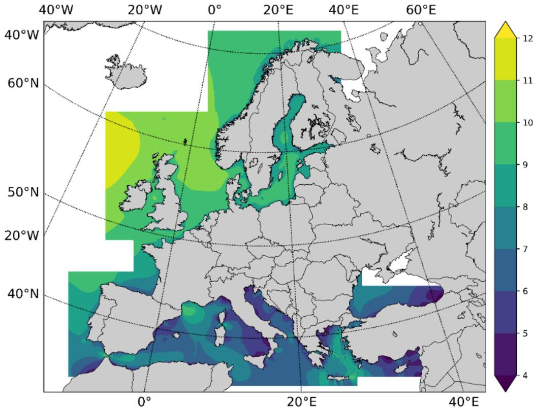
**Figure 4: WRF New European Wind Atlas production run mean wind speed (m/s) at 100m height for 1989 to 2018 with 3 km spatial resolution.**
