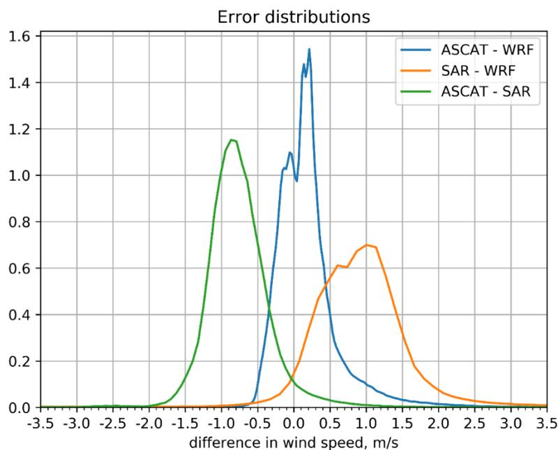
Figure 7: Wind speed difference error distribution at 100m height ASCAT minus WRF, SAR minus WRF and ASCAT minus SAR.
