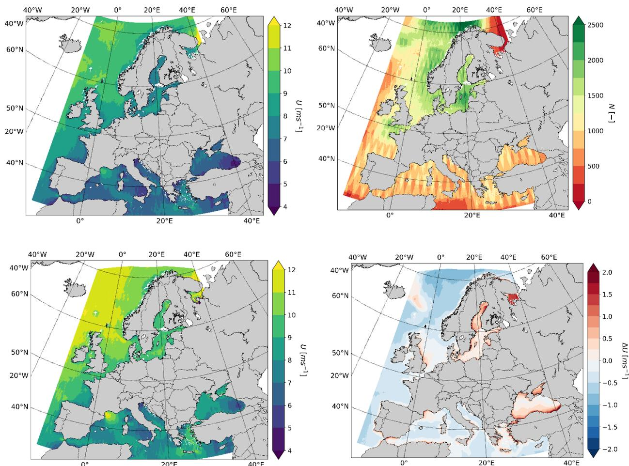
**Figure 3: Envisat ASAR and Sentinel-1 combined: Mean wind speed (m/s) at 10m height (top left), number of samples (top right), mean wind speed at 100m including long-term stability correction for extrapolation (bottom left) and difference on wind speed at 100m height based on long-term stability correction minus neutral wind profile assumption (bottom right).**
