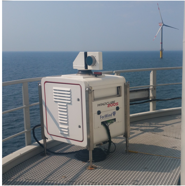
Figure 3. Lidar system Windcube200S on the transition piece of wind turbine GT58 in the offshore wind farm «Global Tech I». On the right side of the image the tower of the turbine is visible while turbine GT51 northwest of GT58 can be seen in the background (c.f. GTI layout in Figure 2). (Stephan Voß, ForWind)
