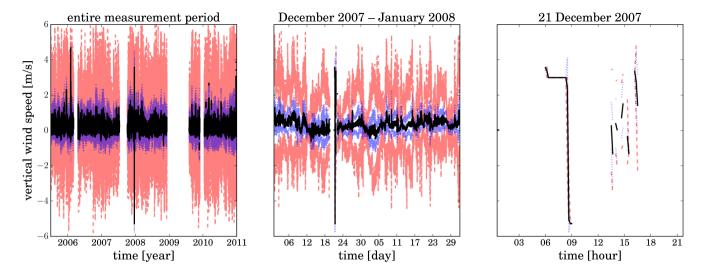
**Figure 2.** An illustration of the visual inspection and zooming of plots. We present the OWEZ vertical wind speed data collected by the ultrasonic anemometer at the NE-116 m location. (Mean in black; mean  $\pm$  standard deviation in blue; minimum and maximum in red.)
