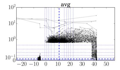
**Figure 6.** Illustrative plots for visually identifying outliers : FINO(cf. pages 1-9-11 for an explanation): FINO1 72 m ambient temperature data [°C].
