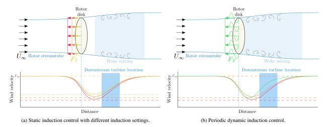
Figure 1. A schematic representation of the streamtube of a turbine, for different axial induction settings. The velocity profile with respect to inflow velocity  $U_{\infty}$  is shown on the bottom, with in blue the area of interest where a downstream turbine is typically located.
