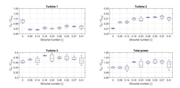
Figure 10. A boxplot showing the variance of the  $C_P$  measurements for the low turbulent,  $C'_T = 1$  experiments, for all turbines individually as well as for the entire wind farm. The f = 0 measurement represents the baseline case of no dynamic control.
