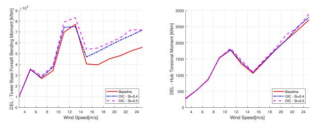
Figure 8. Comparison between tower base fore-aft bending moment (left) and hub torsional moment (right) DEL of the baseline (solid red) and DIC with St=0.4 (dash-dotted blue) and St=0.5 (dashed magenta) as functions of wind speed. Space before unit in xlabel
