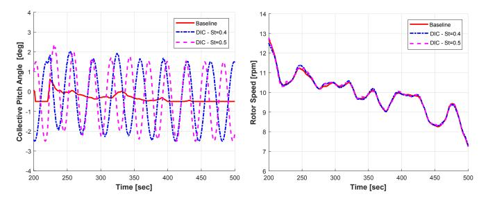
Figure 5. Comparison of pitch activity (left) and rotor speed (right) between baseline (solid red) and DIC controlled with St = 0.4 (dash-dotted blue) and St = 0.5 (dashed magenta) turbine for NTM class "A" at 9 m/s.
