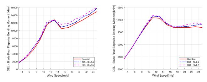
Figure 7. Comparison between blade root flap-wise (left) and edge-wise (right) DEL of the baseline (solid red) and DIC with St = 0.4 (dash-dotted blue) and St = 0.5 (dashed magenta) as functions of wind speed.
