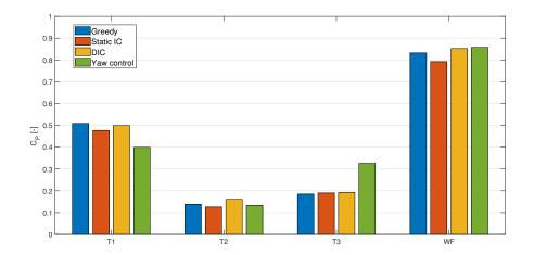
**Figure 12.** The power capture of three state-of-the-art control approaches compared with periodic DIC in low TI conditions. The power capture of the three individual turbines (T1-3), as well the total wind farm (WF) is shown.
