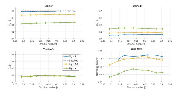
Figure 9.  $\bar{C}_P$  of the wind farm in low TI conditions for different amplitudes of  $C'_T$ . The bottom right figure shows the total power conversion compared to the baseline case.
