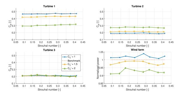
Figure 11.  $\bar{C}_P$  of the wind farm for different amplitudes of  $C'_T$  in the high TI case. The bottom right figure shows the total power conversion compared to the baseline case.
