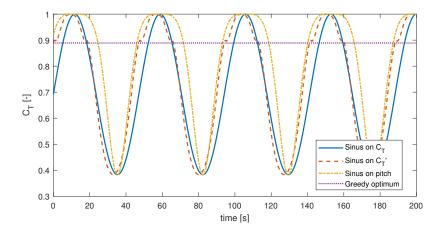
Figure 2. Values of  $C_T$  using a sine-like  $C_T'$  signal with amplitude A = 1.5, compared to a sine on  $C_T$  resulting in a similar amplitude. The dashed line shows the steady-state optimal  $C_T$ .
