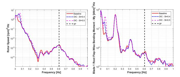
Figure 6. PSD comparison of the rotor speed (left) and blade root flap-wise bending moment (right) between baseline (solid red) and DIC controlled with St = 0.4 (dash-dotted blue) and St = 0.5 (dashed magenta) turbine for NTM class "A" at 15 m/s.
