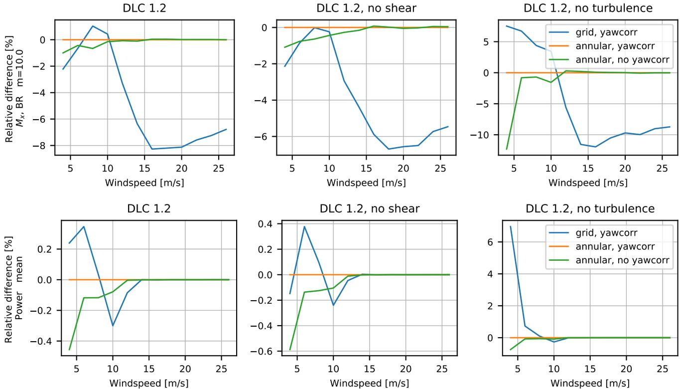
**Figure 18.** A comparison for the DTU 10 MW RWT of difference in blade root flapwise fatigue loads (top row) and mean power production (bottom row) for DLC 1.2 between the ~~annual~~ annular mean BEM method with and without yaw correction and the grid BEM version with yaw correction.
