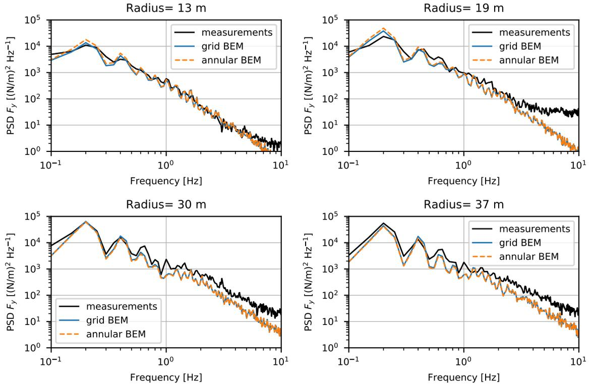
**Figure 24.** A comparison of HAWC2 simulations on the NM80 turbine and experimental results from the DanAero project. Power spectra of the chordwise aerodynamic force component parallel to the chord in comparison with measured results. Wind speed  $6.1 \text{ m s}^{-1}$ , negligible shear and  $\text{rpm} = 12.3$ . Figure reproduced from (Madsen et al., 2018) and adding the annular mean BEM results.
