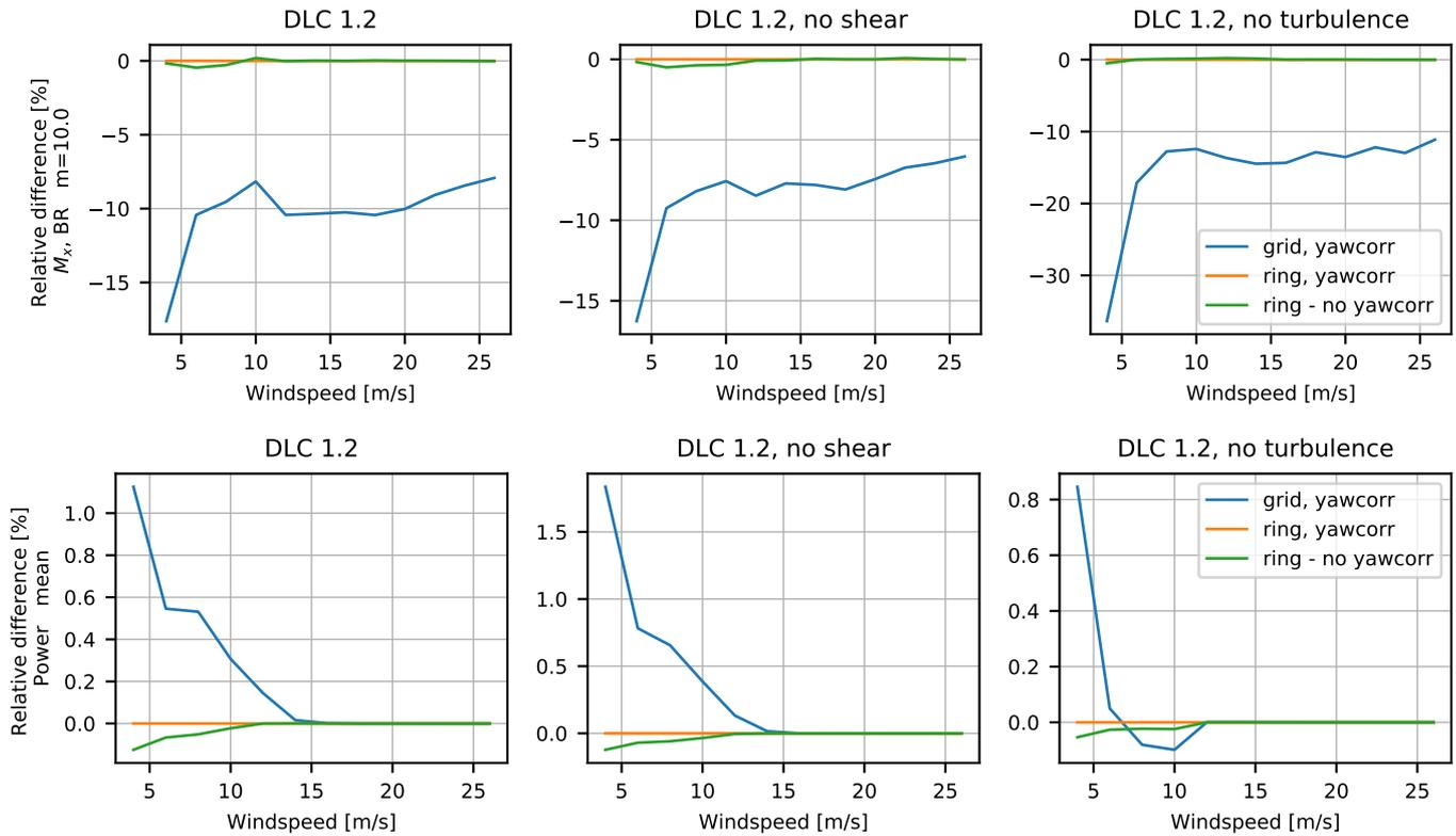
**Figure 19.** A comparison for the AVATAR turbine of difference in blade root flapwise fatigue loads (top row) and mean power production (bottom row) for DLC 1.2 between the ~~annual~~ annular mean BEM method with and without yaw correction and the grid BEM version with yaw correction.
