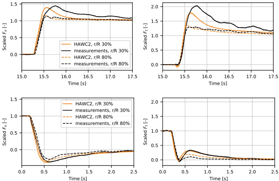
**Figure 27.** Comparison of HAWC2 results against measurements of the dynamic inflow case Q0500000 of the NREL/NASA Ames Phase VI experiment. The plots show scaled normal (left) and tangential (right) forces for pitch steps towards high loading (top) and low loading (bottom).
