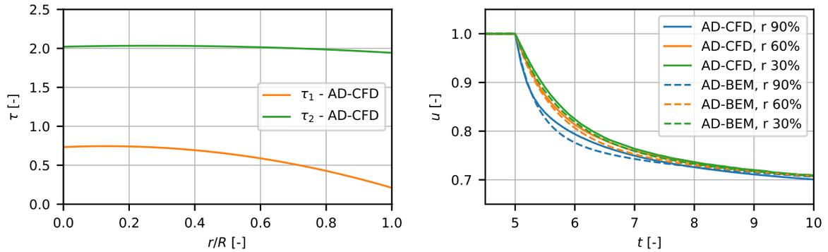
**Figure 11.** Left: Figure showing the derived time constants as a function of non-dimensional radius. Right: Comparison of the step response of the model using tuned constants with the AD-CFD simulations.
