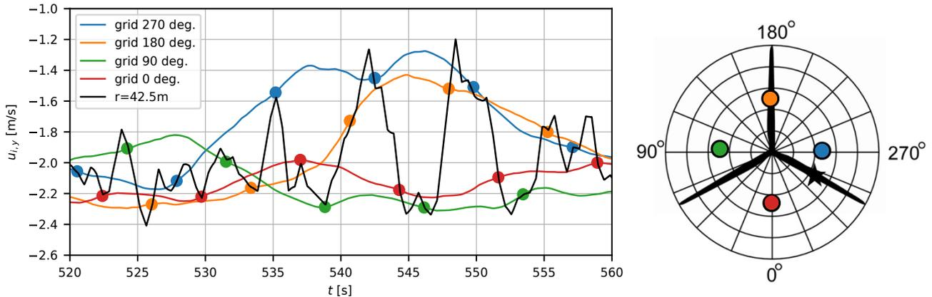
**Figure 14.** Illustration of the dynamic induction mechanism in turbulent inflow showing the blade scanning through the field of slow varying induction velocities but transferring to higher frequencies due to the rotational sampling of the turbulence.
