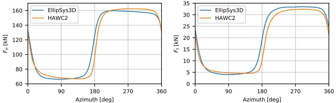
**Figure 23.** Left figure: A comparison of the normal force  $F_n$  as function of azimuth computed with CFD and BEM, respectively. Right figure: Same comparison for the tangential force  $F_t$ .
