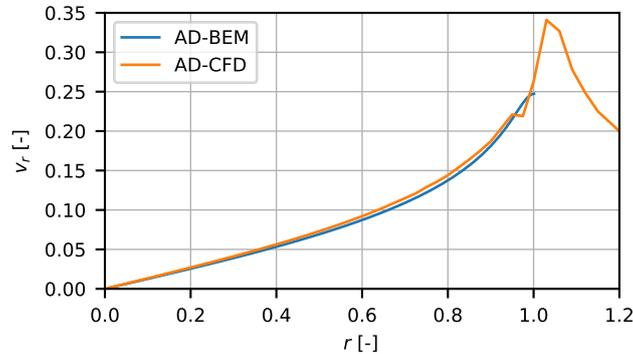
**Figure 13.** The radial induction computed with an engineering sub-model in comparison with AD-CFD result for a constant loading with a thrust coefficient of 0.89.
