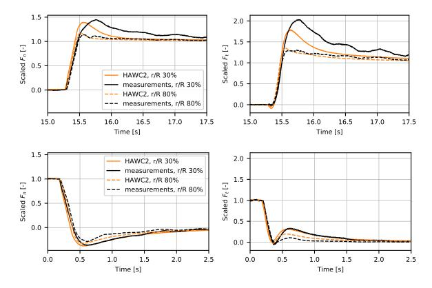
**Figure 27.** Comparison of HAWC2 results against measurements of the dynamic inflow case Q0500000 of the NREL/NASA Ames Phase VI experiment. The plots show scaled normal (left) and tangential (right) forces for pitch steps towards high loading (top) and low loading (bottom).
