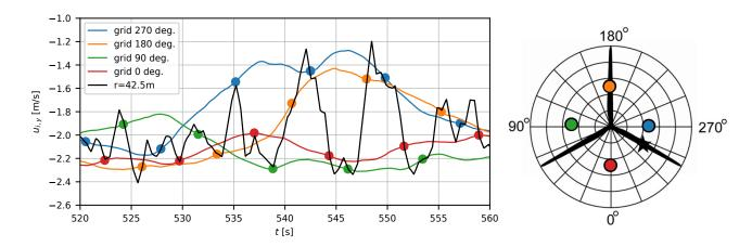
**Figure 14.** Illustration of the dynamic induction mechanism in turbulent inflow showing the blade scanning through the field of slow varying induction velocities but transferring to higher frequencies due to the rotational sampling of the turbulence.
