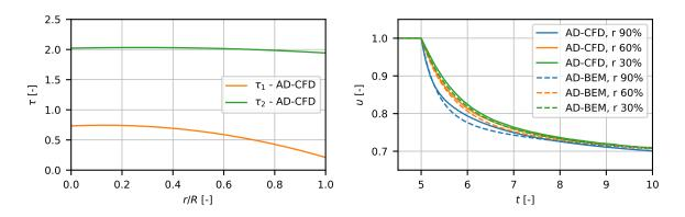
**Figure 11.** Left: Figure showing the derived time constants as a function of non-dimensional radius. Right: Comparison of the step response of the model using tuned constants with the AD-CFD simulations.
