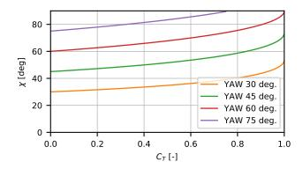
Figure 7. The wake skew deflection angle  $\chi$  against the thrust coefficient for different yaw angles. For zero loading the angle is equal to the yaw angle, whereas the deflection angle increases in combination with an increased thrust level on the turbine.
