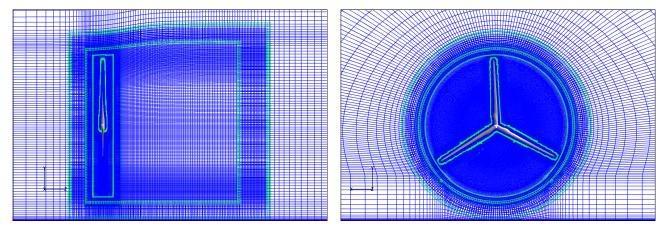
Figure 20. Side-view and front-view of the CFD mesh around the NREL 5 MW reference turbine generated with a hub height of 90 m.
