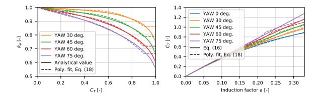
**Figure 5.** Left: Figure showing the reduction factor of the induction a as function of  $C_T$  for different yaw angles. Right: Relation between the thrust coefficient  $C_T$  and the induced wind speed factor a in yawed inflow.
