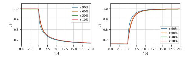
**Figure 10.** The response of the axial velocity to a step change in loading at the actuator disc at different radial position. In the left is the response with  $C_T$  from 0.0 to 0.89, in the right is the response with  $C_T$  from 0.89 to 0.0. The step change of loading is at t=5.
