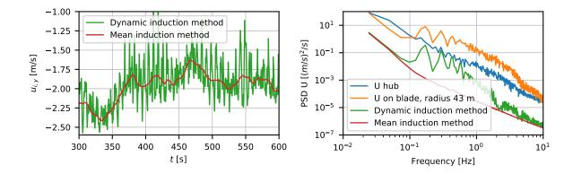
**Figure 15.** Left figure: Time traces of induced velocity at radius 43 m simulated with the annular mean and grid BEM method. The right figure shows the PSD of the same two traces. Additionally in the same figure the PSD of the free wind speed relative to the blade at the same radial position and of the hub wind speed is shown.
