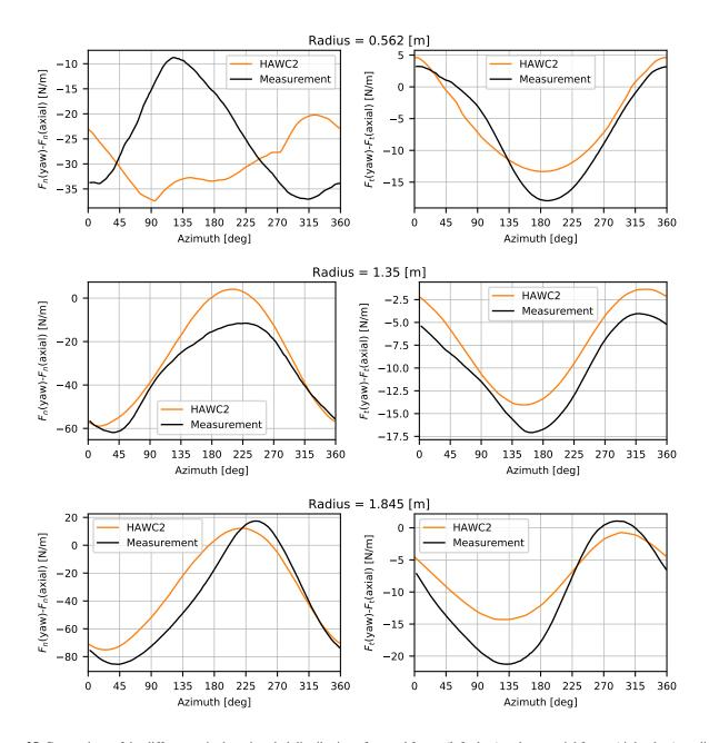
**Figure 25.** Comparison of the differences in the azimuthal distribution of normal forces (left plots) and tangential forces (right plots) predicted by HAWC2 with the forces measured in the New MEXICO experiment, at three different radial positions.
