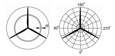
**Figure 4.** Illustration of the BEM approach. Left: Classic approach using an annular element to which the load is assumed constant over the element (mean value of blade forces). Right: New induction grid with annular elements and further subdivided azimuthally
