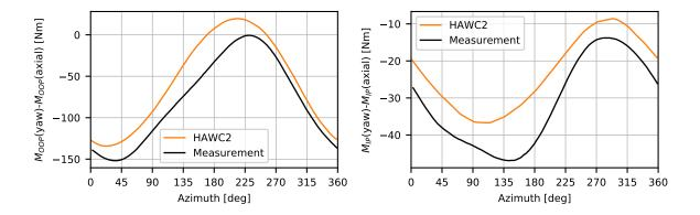
**Figure 26.** Comparison of differences in out-of-plane (left plot) and in-plane blade root bending moments (right plot) predicted by HAWC2 with the moments integrated from the measured forces in the New MEXICO experiment.
