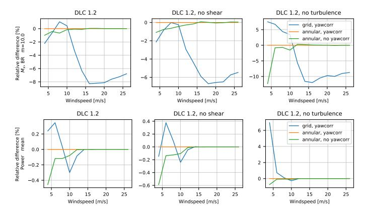
**Figure 18.** A comparison for the DTU 10 MW RWT of difference in blade root flapwise fatigue loads (top row) and mean power production (bottom row) for DLC 1.2 between the annual mean BEM method with and without yaw correction and the grid BEM version with yaw correction.
