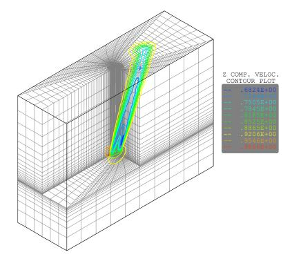
**Figure 2.** The CFD mesh used for the AD yaw computations. The velocity contours for computation of a 30° yawed case is shown on top of the mesh plot.
