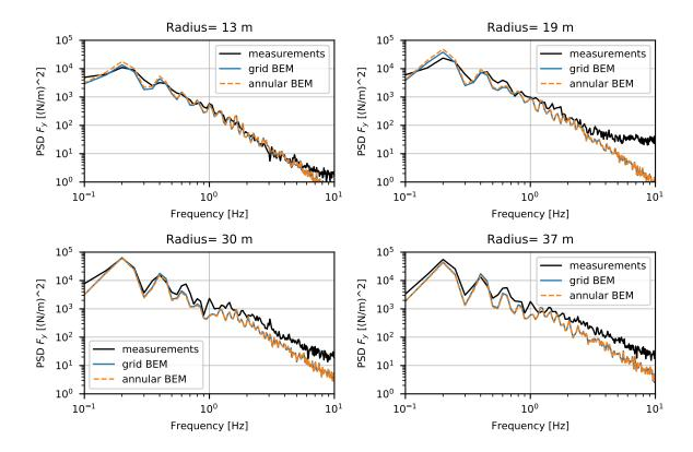
**Figure 24.** A comparison of HAWC2 simulations on the NM80 turbine and experimental results from the DanAero project. Power spectra of the chordwise aerodynamic force component parallel to the chord in comparison with measured results. Wind speed  $6.1 \text{ m s}^{-1}$ , negligible shear and rpm = 12.3. Figure reproduced from (Madsen et al., 2018) and adding the annular mean BEM results.
