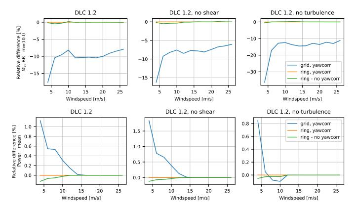
**Figure 19.** A comparison for the AVATAR turbine of difference in blade root flapwise fatigue loads (top row) and mean power production (bottom row) for DLC 1.2 between the annual mean BEM method with and without yaw correction and the grid BEM version with yaw correction.
