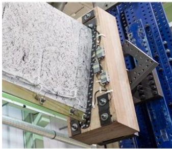
(a) Load frame for blade subcomponent test
