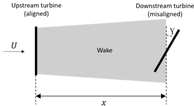
**Figure 3.** Wind turbine layout used in analysis.
