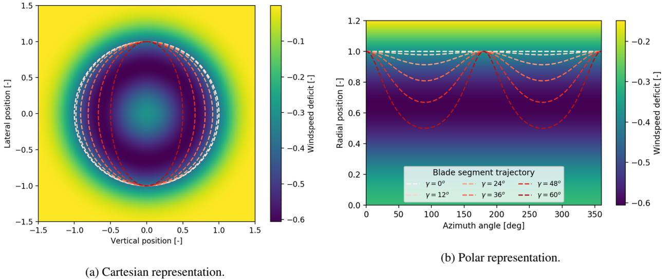
**Figure 1.** The trajectory of a blade segment through a wake inflow at varying yaw angles, represented in Cartesian coordinates (a) and unfolded polar coordinates (b). Distances and wind speeds are normalized by rotor radius,  $R$ , and free wind speed,  $U_0$  respectively. (generated using DWM,  $U = 10 \text{ms}^{-1}$ ,  $x = 3D$ ).
