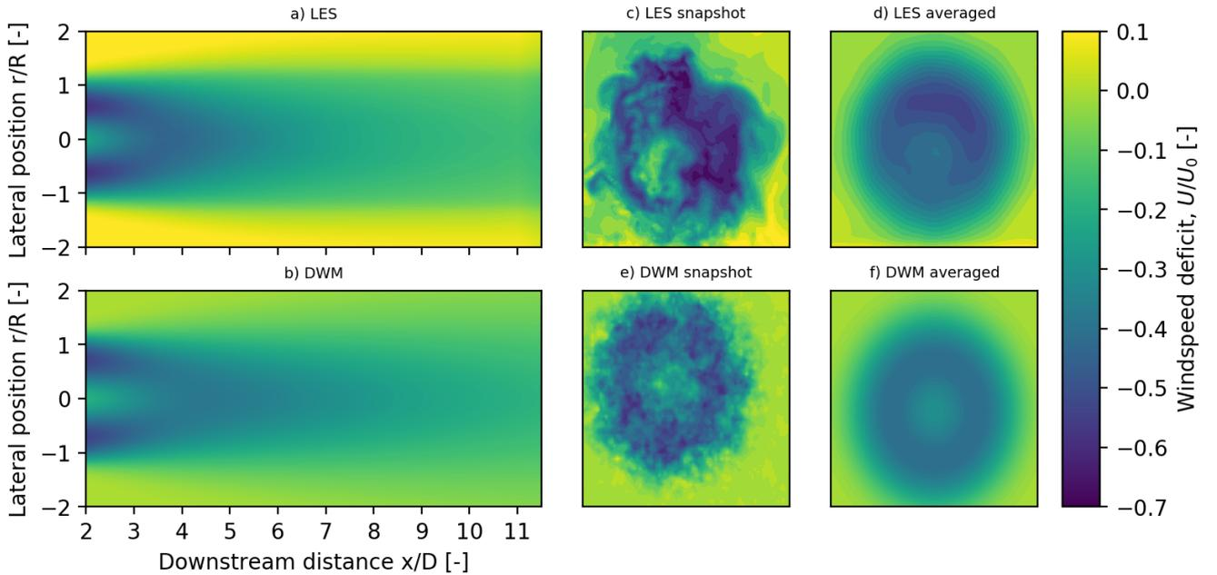
**Figure 4.** Visualizations of the LES and DWM wakes represented as the averaged wake downstream evolution (a, b), wake profile snapshots at  $x = 3D$  (c, e), and wake averaged wake profiles at  $x = 3D$  (d, f).
