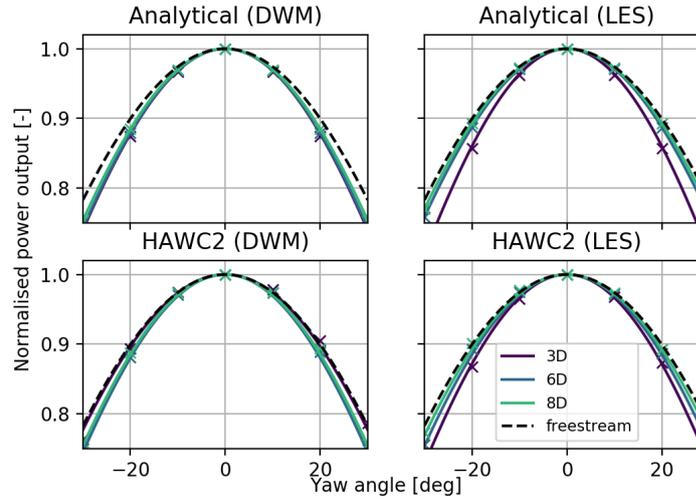
**Figure 5.** Normalized power output as a function of yaw angle for different turbine spacings. Both calculation methods and wake generation tools are presented. The markers indicate the sample points used in the cosine fitting.
