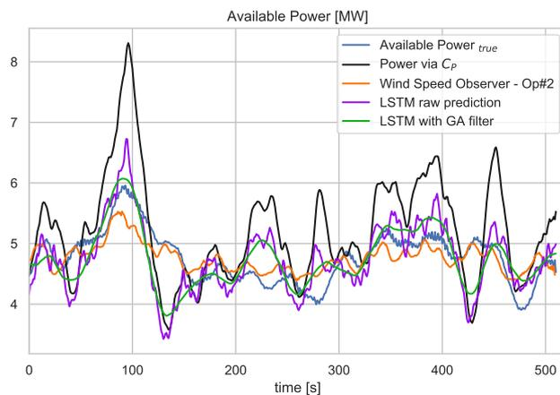
(c) LSTM model results with transfer learning Available Power Estimation (no dependency on level of curtailment). The raw results are presented as well as the post-processing with Gaussian convolution filter.
