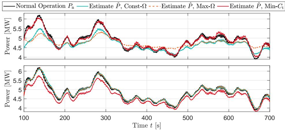
**Figure 2.** Time series of normal power  $P_n$  and available power estimation  $\hat{P}$  based upon various down-regulation strategies. The top and bottom plots indicate the estimation based on measurements of turbines operating at 40% and 80% of the rated power, respectively.
