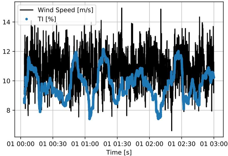
**Figure 13.** LSTM model training with further transfer learning input time series generated by HAWC2, down-sampled to 1-Hz. Mean Wind Speed = 11 m/s, Mean TI = 10%.
