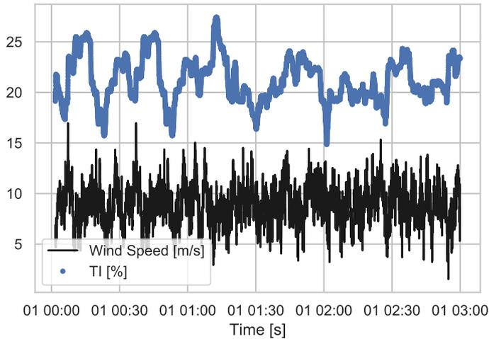
(a) Time series of the inflow dataset for higher TI validation of the transfer learning LSTM model, updated for Mean Wind Speed = 9 m/s and TI = 20%.
