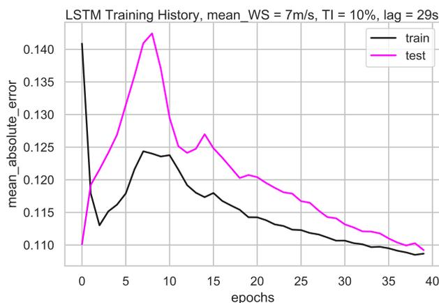
**Figure A1.** Training history of the First LSTM network with mean wind speed = 7 m/s, mean TI = 10%, time lag = 29s. Early stop at 37 epochs due to convergence. The network architecture is presented in Figure 5, batch size = 60
