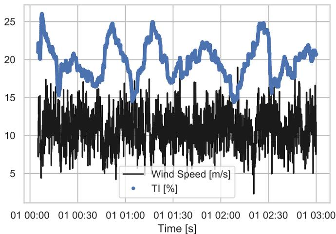
(a) Time series of the inflow dataset for higher TI validation of the further transfer learning LSTM model, updated for Mean Wind Speed = 11 m/s and TI = 20%.
