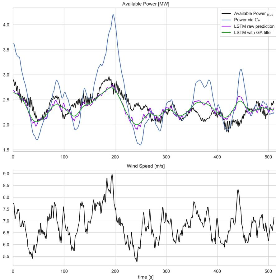
(a) 1-Hz time series of available power and wind speed for the First validation case.
