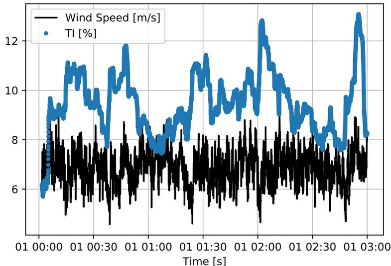
**Figure 4.** First LSTM model training input time series generated by HAWC2, down-sampled to 1-Hz. Mean Wind Speed = 7 m/s, Mean TI = 10%.
