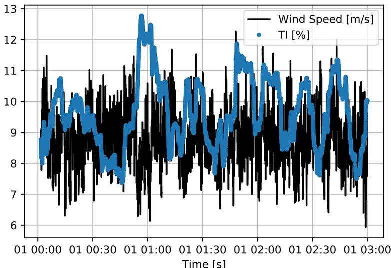
**Figure 7.** Second LSTM model training input time series generated by HAWC2, down-sampled to 1-Hz. Mean Wind Speed = 9 m/s, Mean TI = 10%.
