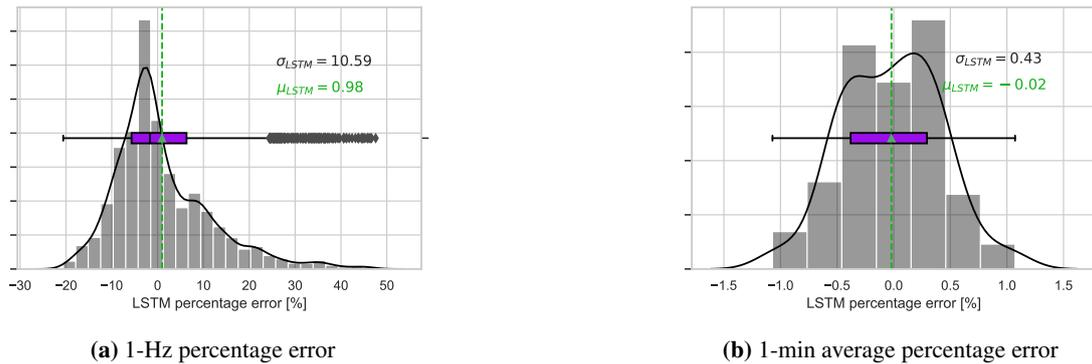
**Figure 14.** LSTM model with Gaussian convolution filter prediction error for further transfer learning flow case. Mean Wind Speed = 11m/s and TI = 10% over 60-min validation case. (a) 1-Hz prediction error, (b) 1min average prediction error.
