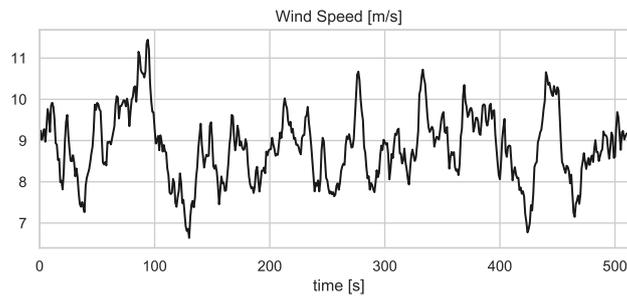
(b) 1-sec wind speed time series for mean wind speed = 9 m/s and mean TI = 10% validation case.
