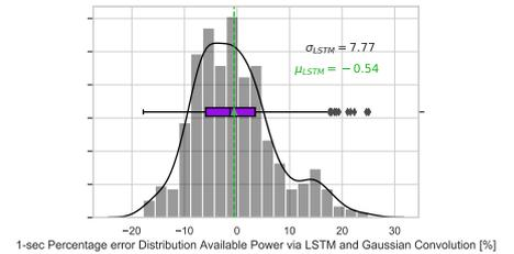
(d) Error distribution of the First LSTM model, with Gaussian convolution.
