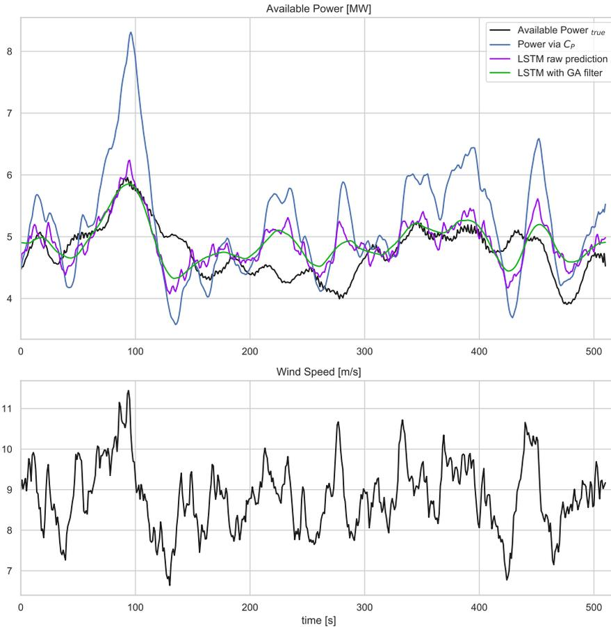
(a) 1-Hz time series of available power and wind speed for the Second validation case.
