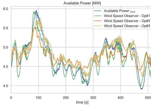
(a) Wind Speed Observer Available Power Estimation for 40% down-regulation case under 3 different curtailment strategies Op#1, Op#2, Op#3. Op#1 with constant rotational speed, Op#2 with maximum rotational speed and Op#3 follows minimum  $C_t$  of DTU 10MW turbine.
