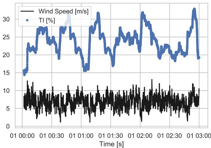
(a) Time series of the inflow dataset for higher TI validation of First LSTM model, trained on Mean Wind Speed = 7 m/s and  $TI = 20\%$ .
