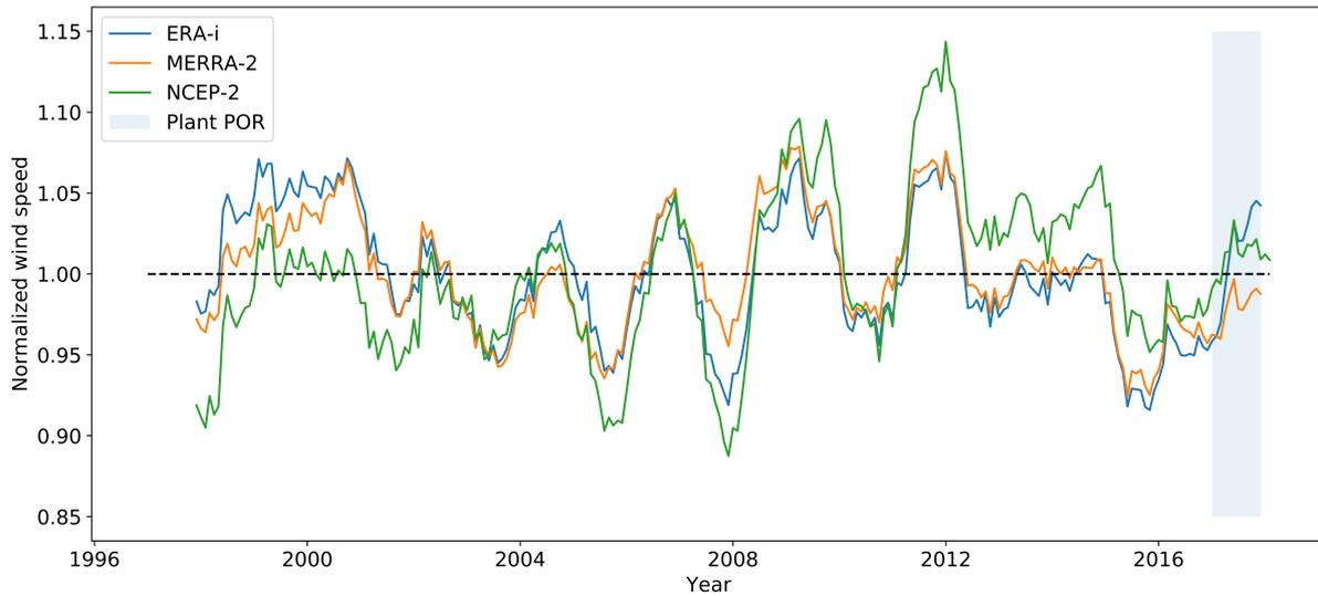
**Figure 8.** Long-term time series of normalized wind speed for EIA station ID 60502 from the three reanalysis products used in the study. The period of record (POR) for the wind farm-plant is highlighted in light blue.
