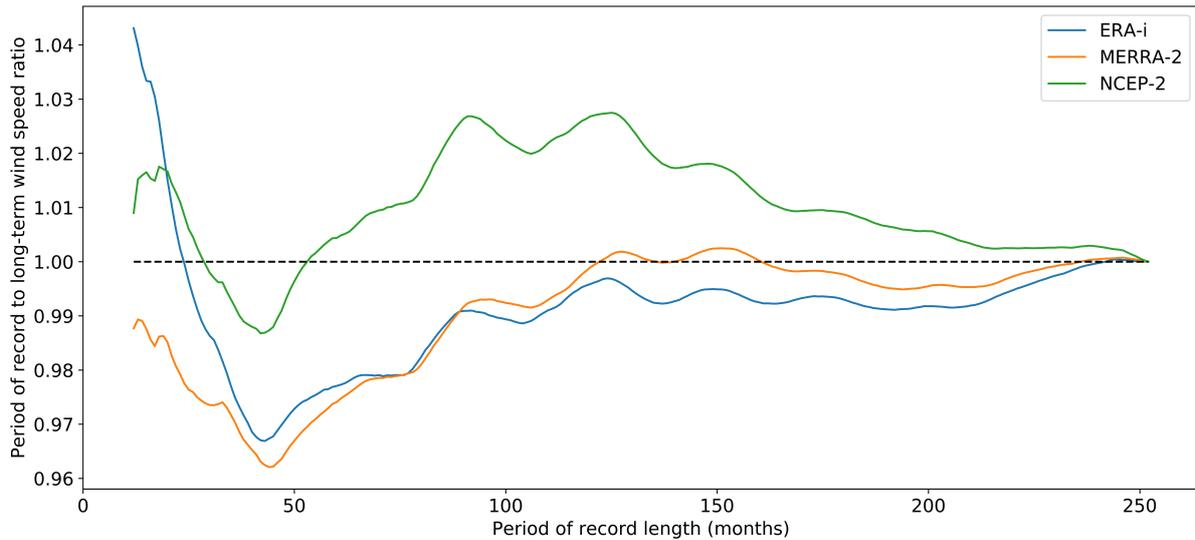
**Figure 9.** Ratio of wind speed to the long-term, 20-year average for periods of record of different lengths (all ending in December 2017), for EIA station ID 60502, using data from the three reanalysis products in the study.
