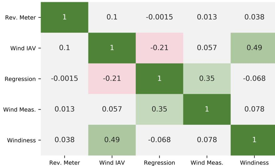
**Figure 6.** Correlation coefficient heat map between operational AEP uncertainty components, as calculated from the results of the Monte Carlo approach applied at the 472 wind farms-plants considered in the analysis. Note: “Rev.” denotes “Revenue”.
