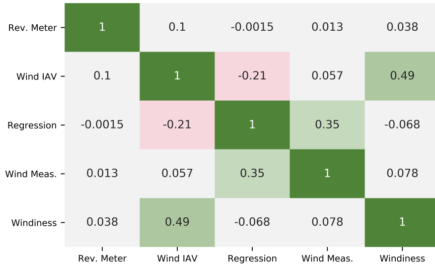
Figure 6. Correlation coefficient heat map between operational AEP uncertainty components, as calculated from the results each pair of the Monte Carlo approach applied at AEP uncertainty components across the 472 wind plants considered in the analysis. Note: “Rev.” denotes “Revenue”.
