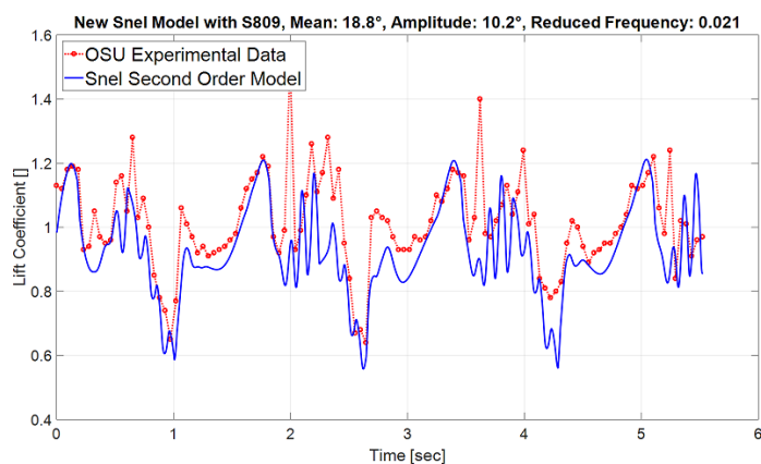
Figure 11: Lift coefficient over time of the improved Snel model (S809 Airfoil at low reduced frequency)
