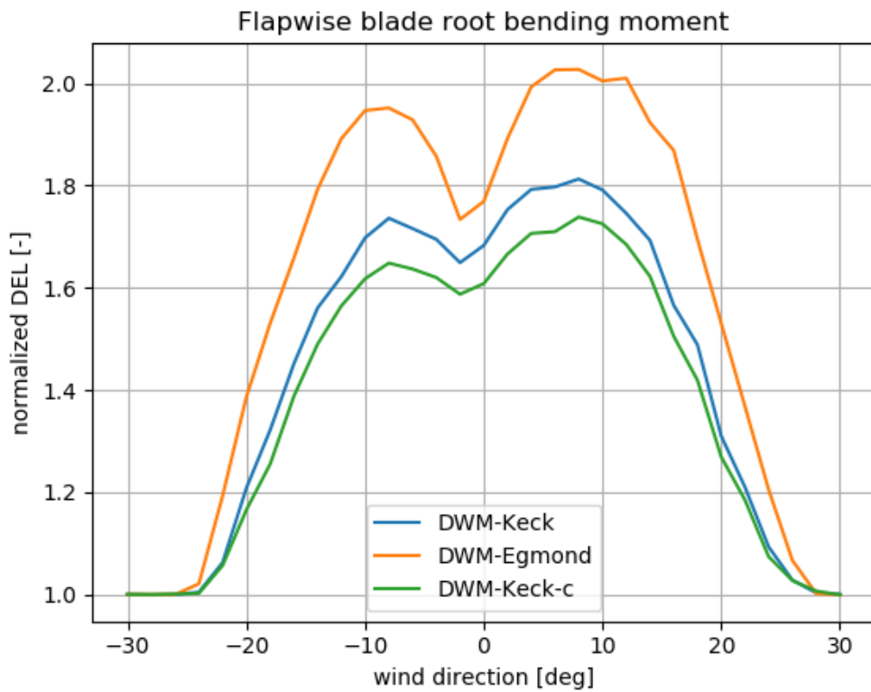
Figure 3: Normalized flapwise blade root DEL over different wind directions for an ambient wind speed of 8 m/s, an ambient turbulence intensity of 12 % and a downstream distance of 3.61D. The DELs have been calculated with a wöhler coefficient of 10.
