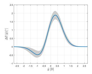
Figure 8. Identified wind direction change  $\Delta\Gamma$  due to secondary steering as a function of distance  $\tilde{y}$  to the wake centerline for a turbine misalignment of  $20^{\circ}$ . The grey shaded area shows the uncertainty band.
