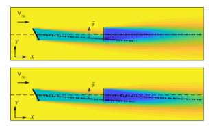
**Figure 1.** Effect of secondary steering on the trajectory of a downstream turbine. Top subplot: baseline wake model; lower subplot: baseline model augmented with the empirical correction term of Eq. (5).
