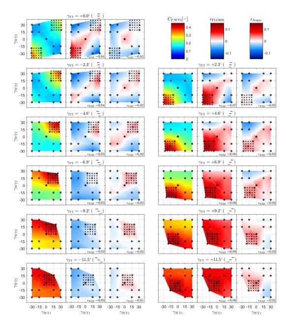
Figure A3. Wind turbine WT3. Each cluster of three subplots represents a unique turntable position, as indicated by the title and the wind farm layout sketch. Left subplot: turbine power coefficient  $C_{P,WT3}$  as a function of  $\gamma_{WT1}$  (x-axis) and  $\gamma_{WT2}$  (y-axis). Middle subplot: FLORIS model error. Right subplot: augmented model error. Cross symbols: all measured configurations. Circles: conditions used for parameter identification.
