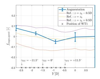
Figure 7. Identified non-uniform inflow speed augmentation term (solid line) and associated standard deviation (whiskers). Hot wire measurements at different heights above the floor are shown in thin solid lines. The upstream turbine (WT1) y position for all investigated turntable rotations is shown by x markers for all investigated turntable positions placed along the lower edge of the figure.
