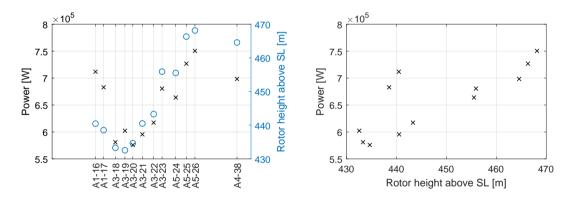
Figure 14. Correlation between power output and hub height with respect to SL. Left subplot: power ( $\times$  symbols and left y axis) and rotor height above SL ( $\circ$  symbols and right y axis) vs. lateral turbine position for a wind direction  $\Gamma = 240^{\circ}$ . Right subplot: power vs. rotor height above SL for  $\Gamma \in [220^{\circ}, 275^{\circ}]$  and  $V_{\infty} \in [8, 10]$  m/s. All conditions are free-stream and all turbines of type GE1.5s.
