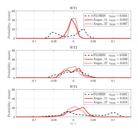
**Figure 10.** Error distributions for each turbine for all tested configurations, for the baseline FLORIS model (black dashed line), the 11-parameter augmented model (red solid line) and the 27-parameter augmented model (red dotted line).
