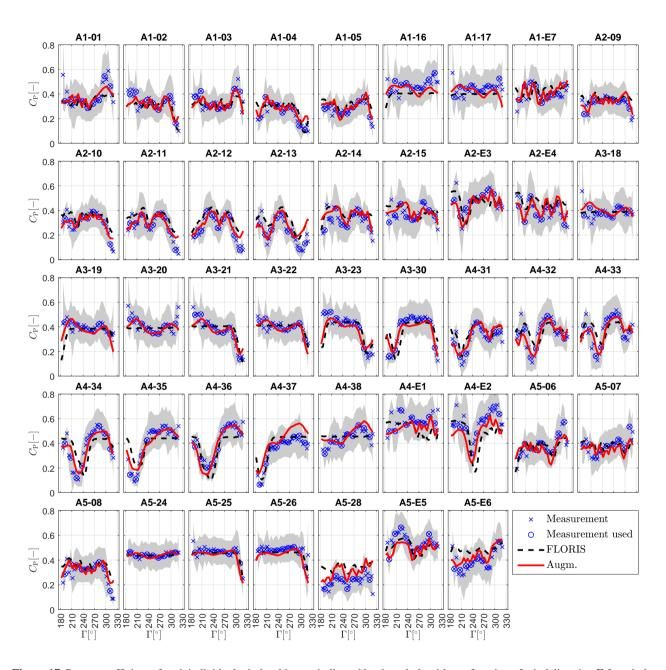
Figure 17. Power coefficient of each individual wind turbine, as indicated by the subplot title, as function of wind direction  $\Gamma$  for wind speeds  $V \in [8,10]$  m/s. The gray shaded area indicates the standard deviation within the binned measurements. The number of measurements within each bin is reported in Fig. 13.
