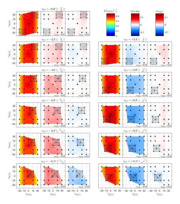
Figure A1. Wind turbine WT1. Each cluster of three subplots represents a unique turntable position, as indicated by the title and the wind farm layout sketch. Left subplot: turbine power coefficient  $C_{P,WT1}$  as a function of  $\gamma_{WT1}$  (x-axis) and  $\gamma_{WT2}$  (y-axis). Middle subplot: FLORIS model error. Right subplot: augmented model error. Cross symbols: all measured configurations. Circles: conditions used for parameter identification.
