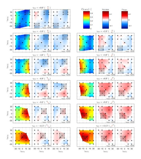
Figure A2. Wind turbine WT2. Each cluster of three subplots represents a unique turntable position, as indicated by the title and the wind farm layout sketch. Left subplot: turbine power coefficient  $C_{P,WT2}$  as a function of  $\gamma_{WT1}$  (x-axis) and  $\gamma_{WT2}$  (y-axis). Middle subplot: FLORIS model error. Right subplot: augmented model error. Cross symbols: all measured configurations. Circles: conditions used for parameter identification.
