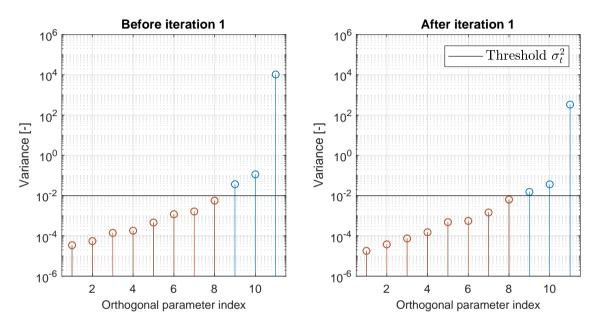
**Figure 6.** Variance of the orthogonal parameters before (left) and after (right) the first iteration. The identifiable orthogonal parameters are shown in red, whereas all others are shown in blue.
