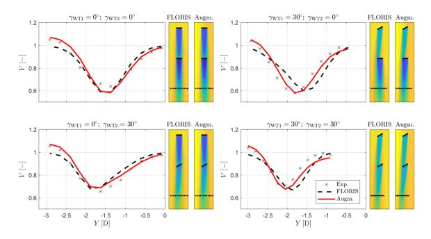
Figure 9. Wake profiles 5D behind WT2 for various combinations of turbine yaw misalignment. Experimental values are indicated by the  $\times$  symbols. Each subplot is accompanied by two flow visualizations based on the FLORIS model and its augmented version.
