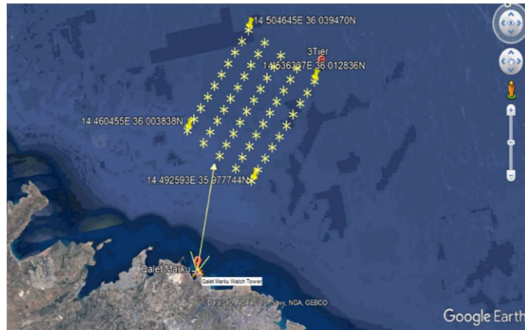
292 293 Figure 6: Satellite imagery of the wind farm showing the location of the 50 wind turbines with respect to the coastal LiDAR 294 station (Google, 2019) (© Google Maps 2019).
