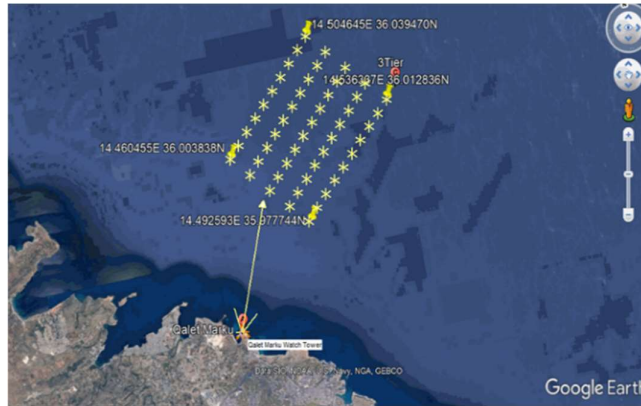
Figure 6: Satellite imagery of the wind farm showing the location of the 50 wind turbines with respect to the coastal LiDAR station (Google, 2019) (© Google Maps 2019).
