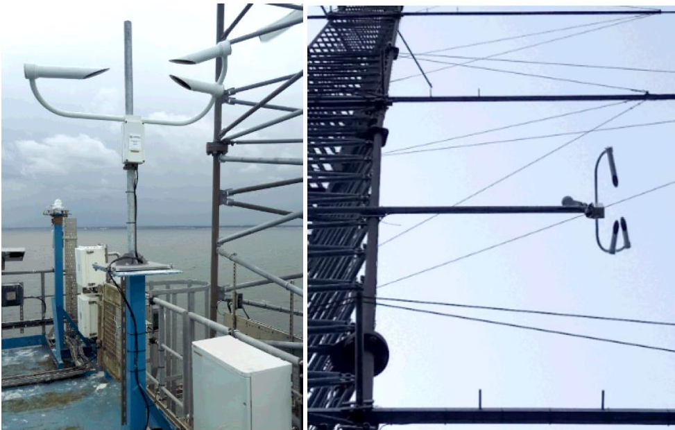
Figure 1: The optical disdrometers mounted to the platform (left) and at 55 m above sea level (right).
