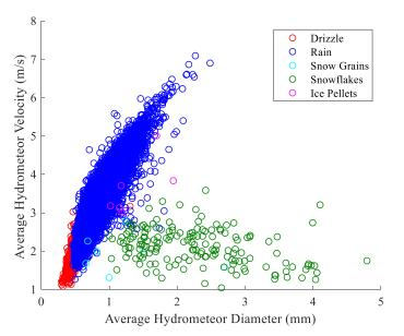
Figure 5: Relationship between size and velocity for the modal hydrometeor at each minute.
