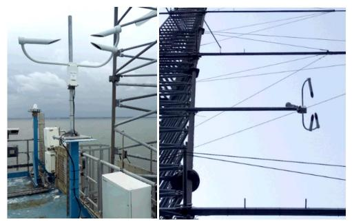
65 Figure 1: The optical disdrometers mounted to the platform (left) and at 55 m above sea level (right).
