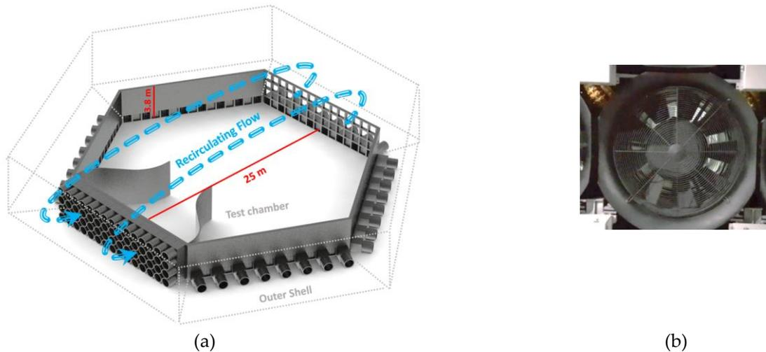
**Fig. 2: WindEEE dome, (a) the test chamber and the contraction walls with the flow recirculation path through the outer shell in closed circuit 2D flow mode, (b) the adjustable vanes at the inlets of the 60 fans at 70% opening vanes state**
