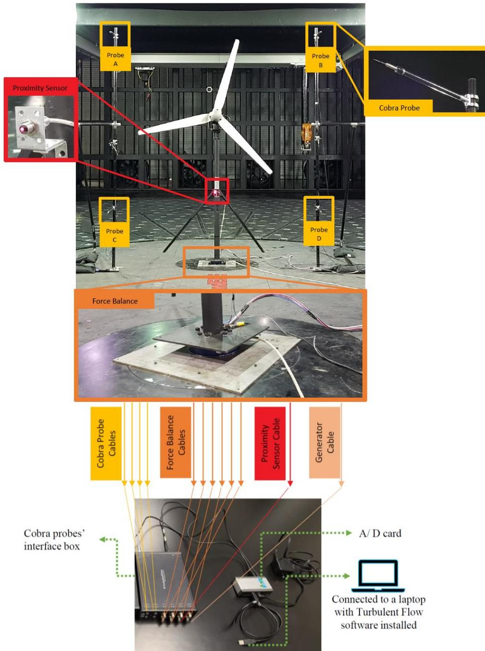
**Fig. 3: Setup for measuring power performance and dynamic loads for different types of inflow**
