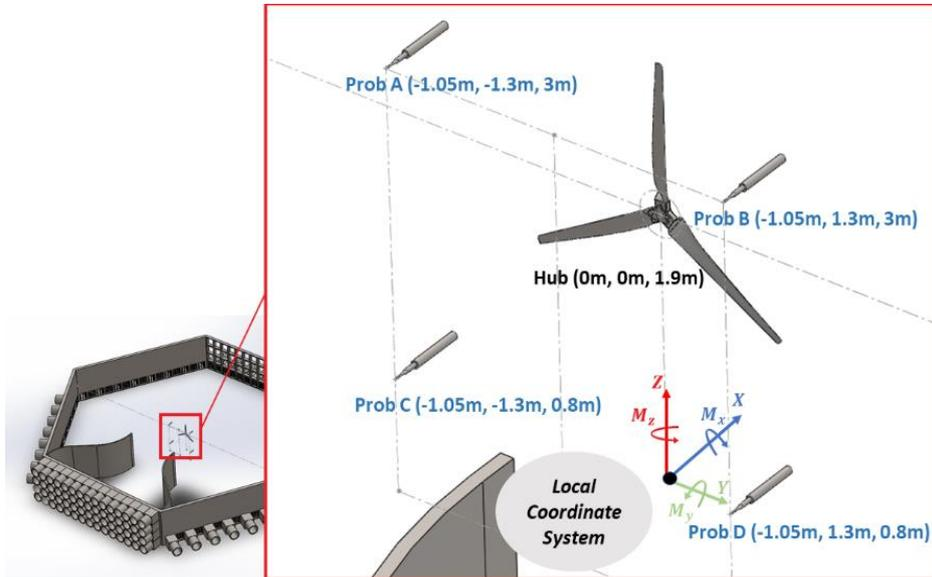
Fig. 4: The arrangement of cobra probes and HAWT relative to local coordinate system
