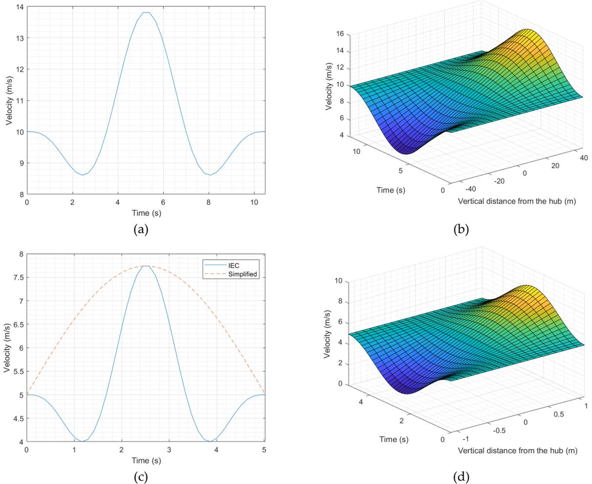
**Fig. 1: Extreme operational conditions for a full scale HAWT  $III_B$  class with 92m diameter and hub height of 80m at 10 m/s uniform wind speed, (a) extreme operational gust, (b) extreme vertical shear on the rotor with hub height as reference, The scaled extreme condition, (c) the IEC EOG and the simplified EOG that was targeted, (d) extreme vertical shear. Adopted from (Shirzadeh et al., 2020).**
