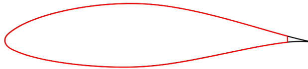
Figure 2. NACA 654-421 profile manufactured in red and the theoretical trailing edge in black
