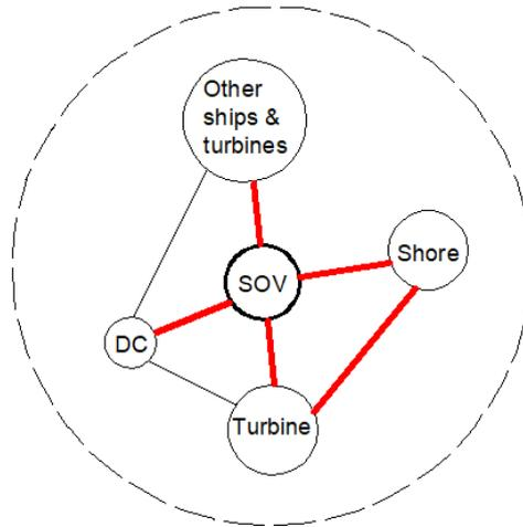
Figure 4: System components and system boundary (SOV – service operation vessel, DC – daughter craft)
