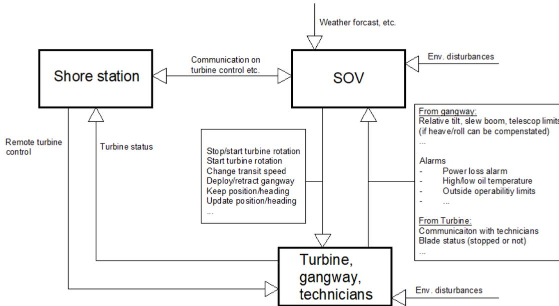
Figure 3: Hierarchical safety control diagram of interface between SOV and turbine (further explained in Section 4.2)
