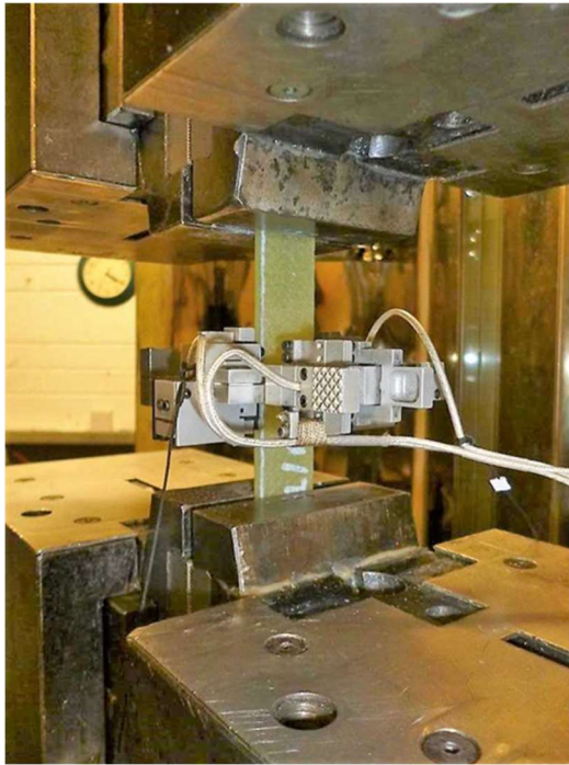
Figure 2: Experimental static testing of glass-fibre reinforced specimens, where (a) is the tests being performed and (b) is a comparison of the experimental static testing results with the results from the FEA model
